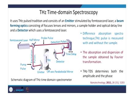
But, let us see what terahertz time domain spectroscopy is. This is spectroscopy which measures actually the absorption spectra with and without the sample from the terahertz pulse. So, what you do is that you measure the absorption and dispersion of the sample by using Fourier transform. It gives you both, I mean, amplitude as well as the phase.
