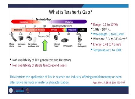
Terahertz gap: now there is a gap; I mean the field of electronics is full fledge developed and the photonics is developed full-fledged, but there is a gap at the juncture, where electronics and photonics meet. Actually, you do not have detectors or sources in this particular range, that is that is why it is called terahertz gap and there are no available femtosecond lasers also.
