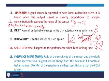
Linearity; a good sensor is expected to have linear calibration. What it means? like I told you that lambda resonance versus C curve and I showed you this kind of thing. Suppose, you have like this it is not linear here.
