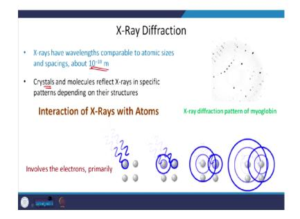
For example, I have shown here X-ray diffraction spectrum of myoglobin and what happens actually that these crystals and molecules reflect X-rays in a specific pattern depending on their structure. If you have an atom, there are basically electrons and it comes and interacts with these electrons. It can either expel it to the outer cells and then again it comes back and gives the radiation. So, it is basically involvement of electrons, when you consider the interaction of X-rays with atoms.
