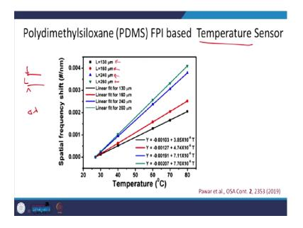
Here I will show you another sensor which is a temperature sensor on similar kind of structure. What you see is that for different thicknesses of this cavity - L is the thickness of the cavity. You can see that for different thicknesses, it shows shift in wavelength that is delta lambda basically and you can see that with an increase in temperature, there is a red shift. That is how you can use it for sensing applications.
