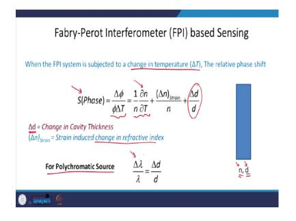
How we use it for sensing that is what we want to focus on. If we have, say a thin film which has refractive index n and thickness d, what can we do - what things can we do? Then here is - either you change the refractive index, or you change the thickness.
