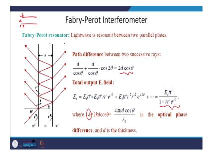
If you see a Fabry-Pérot interferometer, basically this is a thin film which has two mirrors facing each other and when a ray of light enters to it, it gets partially reflected from one boundary and then transmitted through the medium and then again back and forth reflections. We have solved these kinds of equations, if you remember, for one reflection, we solved it for the Fresnel equations.
