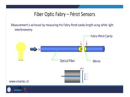
If you want to use fiber optics for Fabry-Pérot sensors, you can have a couple of configurations. One of the configurations is that you place two small pieces of this optical fiber where light can be incident through this end, and it is the polychromatic
