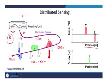
You have the reading unit and you have an optical fiber that is distributed sensor - at 0-meter, 1 meter, 100 meter, 1000 meters, 40 kilometers, you want to sense - say temperature and strain. Suppose, this temperature change occurred somewhere here, you do not know what the distance is. It is also possible then you send a pulse it shows that at this particular position, you have this much change in temperature.
