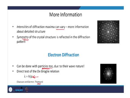
Intensities of diffraction maxima can also vary, and it gives more information about the detailed structure. Suppose sometimes the intensities will also vary and that will give you an exact information, we will come to that. And symmetry of the crystal is also reflected in the diffraction pattern.
