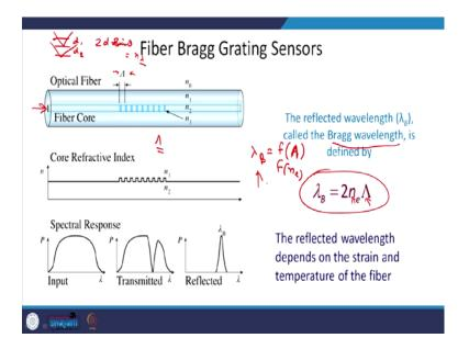
Fiber Bragg grating sensor: We saw Bragg diffraction and there we saw that if you had different layers placed at d 1, d 2, d 3 - something like this and then light comes and strikes like this, then we had this condition - 2d sin theta is equal to n lambda; or maybe you can say n lambda - something like this we saw. Here if you have refractive index, then there will be n term also.
