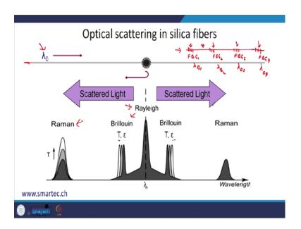
Optical scattering in optical silica fibers: we know that when light travels, say of wavelength a lambda 0, through an optical fiber what will happen that a small part of it will get scattered and back is scattered also. So, the scattered light will be everywhere, and we know that what kind of scattering can there occur. We already talked about Raman; it can also be Brillouin scattering, which is very close to - bands very close to - the incident wavelength.
