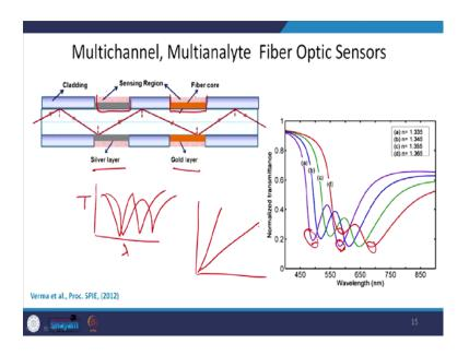
So, what you have to do is that at multiple segments of the optical fiber you make different sensors and then it works as a cascaded sensor or multichannel sensor or you can use it for multi-analyte sensing also. We are taking another example of an optical fiber SPR sensor. We already discussed what is SPR. We also discussed how to excite SPR in a fiber geometries.
