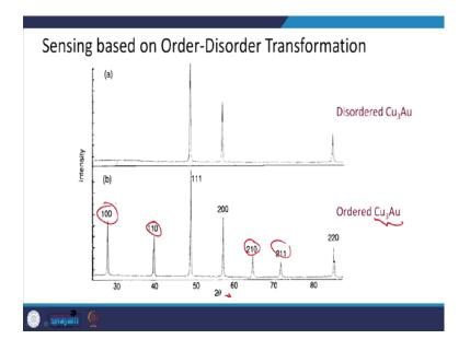
Let us see one case - sensing based on order-disorder transformation. I have this Cu 3 Au molecule, where you can see that for this compound these are the diffracted peak positions as a function of 2 theta. These are the XRD patterns. And when it becomes disordered, then these peaks disappear - you see. So, what it essentially means? It essentially means that you can use it for sensing application.
