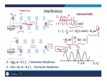
In interference, you know that, if you have two coherent waves and they are superimposed on each other you will get either a maximum or a minimum. Suppose you have an amplifier connected with two speakers and they are producing longitudinal waves like sound. So this travels in the form of compression and rarefaction; these
