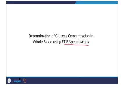
We will show you something called Fourier transform IR spectroscopy. Let us say that our source is in IR and we want to determine the glucose concentration in the whole blood using this technique. So, FTIR technique - what is this? You have an IR source and this IR source is having multiple wavelengths. It is not just one wavelength - it is a broadband source and you have a sample here in (Refer Time: 17:46) one of the arms. What would happen?
