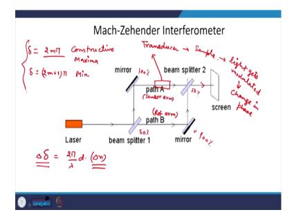
Mach-Zehnder interferometer: In this kind of interferometer, you have two mirrors and two beam splitters. Light goes like this. You have a beam splitter which partially reflects and transmits, the light can go from here and here, then again from - this is 100 percent reflecting, this is say 50 percent reflection, and same here 100 percent and here it is 50 percent reflection. So, what happens actually - That these two beams combine here to give you the interference pattern.
