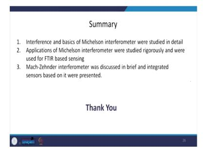
Let us summarize this. We discussed today what is the interference and the basics of Michelson interferometer. Then we studied what are the applications of Michelson interferometer and how can it be used for sensing, and we showed one example of Fourier transform IR sensing. So, Fourier transform spectroscopy - we studied what it is, the basics and then why we are going in IR and then how we are using it for detection of glucose in whole blood.
