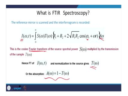
You can move the reference mirror which was this mirror, and you can have I as a function of delta d on that will come in terms of phi naught plus omega t into d omega. So, if you solve for the Fourier transform, you can have Fourier transform of I omega t and normalization to this gives T omega, that is the transmission with respect to omega or in terms of absorption. Because you know intensities, you can always convert it to transmission or reflected or absorption power.
