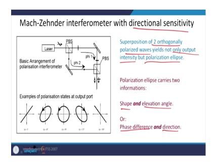
It can also be used with directional sensitivity. Suppose you have now super-position of two orthogonally polarized waves, it will not only change the output intensity, but also the polarization ellipse. Here are two polarizations which are orthogonally polarized and then they are super posed. Polarization ellipse carries two information, one is the shape and other elevation angle - or you can say phase difference and direction. By this way you can have a differential phase in measurements also.
