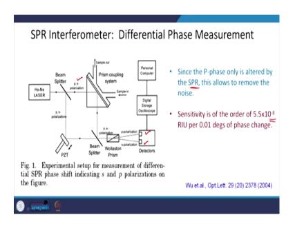
Sensitivity in this particular case is of the order of 10 to the power minus 8 RIU per 0.01 degrees of phase change. So, it is very sensitive.
