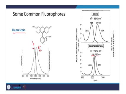
What happens in fluorescence - for example Fluorescein, I have taken this molecule, you shine it with certain light. Here is the absorption curve - it gets adsorbed there. After this kind of vibrational relaxation, it comes down emitting light of wavelength which is larger than the absorption wavelength. This is called fluorescence. This is the absorption plot, this is the fluorescence plot.
