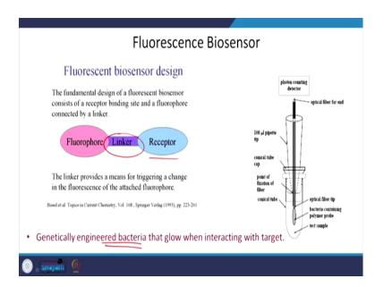
If you want to design a fluorescence biosensor, what to do is that you attach this fluorophore to the receptor via some linker. For example, I have shown here genetically
