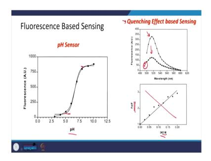
If you want to use them for sensing, for example, what we can do is that we can have a quenching or enhancement-based effect. For example, in this particular case, you had this curve and after you put some molecule the fluorescence got quenched. So, by measuring how much change in intensity occurred, you can see that how much change in concentration occurred there. It can be vice versa also.
