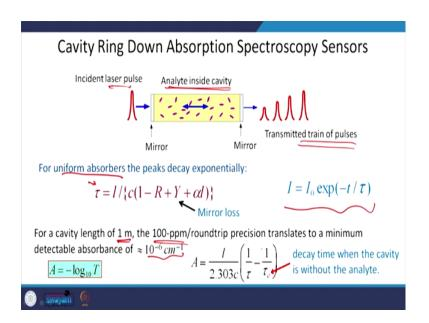
And when a laser pulse is incident in it, it goes, gets absorbed and after back and forth reflections, you have transmitted train of pulses. For uniform absorbers, the peaks decay
