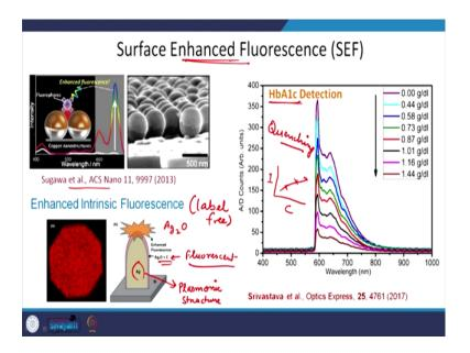
What happens actually is that when you bring an analyte near this receptor, it leads to change in the fluorescence of this. That is why it is called label-based sensing - labeled sensing, because you have to have a fluorescent tag whose intensity changes when there is a bio sensing interaction. If you bring this kind of fluorophore near a metallic nano structured surface - plasmonic surface, then its fluorescence can be enhanced and that is why it is called surface enhanced fluorescence.
