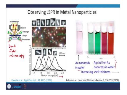
It is done using dark field microscopy. What to do is that this excitation light, which is coming from this direction and this direction does not go into the scattered light direction; you block it somehow and then only the light which is scattered from the nanoparticles is captured by the camera. So, you can see different colors, which are pertaining to different shapes and sizes of the nanoparticles and here you can see that they can correspond to different resonances for different dimensions.
