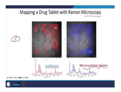
We can map drugs using Raman technique. So, now you can have a Raman microscope integrated to the spectrometer. What you get is an image, a map of the tablet. Suppose you have a tablet here and you take the Raman spectra, Raman images from different places, you can do a mapping and it will tell you what the components of this tablet are.
