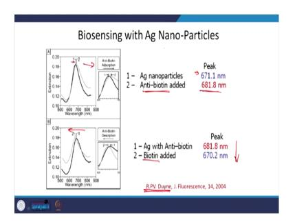
This is work from one of the pioneers of SERS, R PV Duyne, who used silver nanoparticle for biosensing - it just a proof of concept. You can see that in first one is the silver nanoparticles and when you add anti biotin it shows a small shift in the absorption. So, the peak shifts from 671 to 681 nanometers. Similarly, if you have Ag with anti-biotin already and now you add biotin it will again show a shift.
