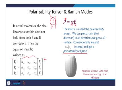
However, it is very useful technique. What happens actually - you have a molecule and you are incident with an electric field- you already know this thing that what happens that it gets polarized. The electric field is in this direction you will have a dipole in this direction, the electric field of the dipole will be in other direction. So, it will be polarized and the dipole moment will be given by polarizability of the molecule into the electric field.
