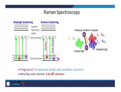
Now, let us see what Raman spectroscopy is and how we can use it in conjunction with localized surface plasmons to make very highly sensitive sensors. We know that if you have a molecule and we shine with a laser, most of the light which gets scattered from
