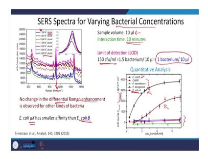
So, what we see? Here we have shown the SERS spectra for varying bacterial concentrations and you can see that if we increase the bacterial concentration say from 1.5 into 10 to power 2 colony forming units per ml - like 150 bacterial cells per ml to about 3 into 10 to power 5 bacterial cells per ml, you get this spectra. You cannot determine what is happening here.
