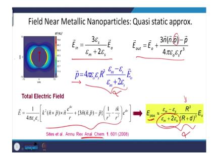
When we solved the Laplace equation and we arrived to the potentials, and then we derived from there the electric fields inside and outside the nanoparticle, we found that it has a dipole term, and that dipole was given by this term, where you can see that this is polarizability - if you remember, alpha, and the total electric field can be written as E inside plus outside, which is given by this relation. You can find its rigorous derivation in various reviews.
