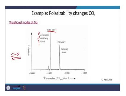
You see the vibrational modes of carbon dioxide and the symmetric stretching mode is given by this at 1388 and bending mode is here. So, even if it was carbon - oxygen bond, different vibrational modes will give you different frequencies - that is how you characterize these molecules, ok. Raman spectroscopy can be used to stop fraud.
