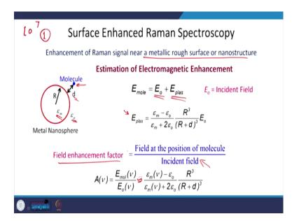
Now, as I told you that, out of 10 million photons -10 to the power 7 photons, only one gets Raman scattered. It was found that if you bring this molecule, which you want to study for Raman spectroscopy - if you bring this close to a metallic rough surface or a metallic nanostructure, you can enhance the Raman signal. Why? Because of plasmons. We already know that in the vicinity of the plasmonic structure you have enhanced electromagnetic fields.
