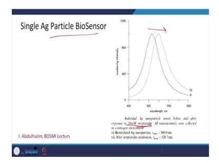
You can have single silver particle biosensors, so on one single nanoparticle before and after exposure of 10 nanomolar streptavidin you can see that a shift of about 13 nanometers occurs by adding streptavidin. So, that is how you use nanoparticles for localized surface plasmon resonance space sensing.
