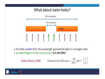
Now, what will happen if I make all this nanometer sized - say about 20 nanometer hole in a 100 nanometer film? Is it still 20 percent? Now, remember we have holes which are smaller than the wavelength of light - 20 nanometer hole. In 1944, Bethe predicted that the transmission efficiency of such kinds of structures is inversely proportional to lambda. So, if you have r much smaller, the transmission efficiency will be 0, practically 0; it has to be 0, that is what he predicted ok.
