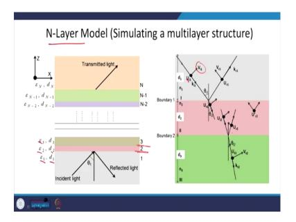
Today we will solve it using matrix method and it is very easy to solve. What we do is - we consider a N layer model - we want to simulate a multi-layer structure. So, suppose we have N layers of reflective indices say epsilon 1, epsilon 2, epsilon 3, so on and the thicknesses of these media d 1, d 2, d 3 and so on. Light is incident in the medium 1, at angle theta 1 and it gets reflected and partially get transmitted after the Nth layer.
