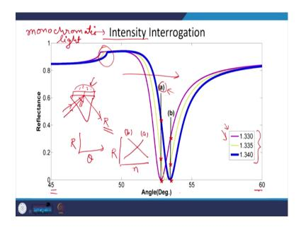
In intensity modulation, you know - I mean, when we plotted the SPR curve - for change in angle with respect to change in reflectance, we saw this kind of dip in reflectance at some angle which was called the angle of resonance.
