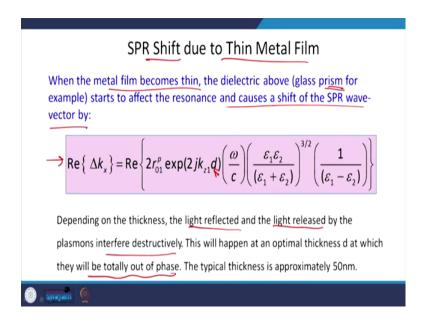
So, let us see what happens. SPR shifts due to this thin metal film. So, what happens that when the metal becomes thin, the dielectric above it starts to affect the resonance and causes a shift to the SPR wave vector. This is the small change in the real part of the wave vector with respect to change in the thickness of the film. So, if you make it thin, say from 50 to 40 nm, there will be a small change in the wave vector and that wave vector is because of the change in the prism layer, ok.
