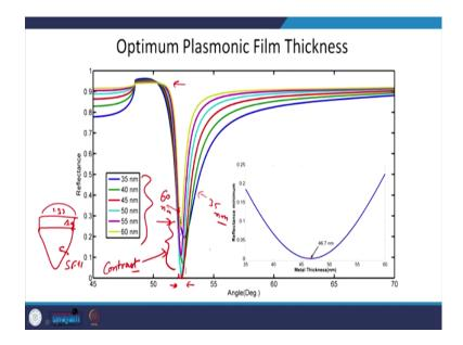
So, here I show you SPR reflection curves for different thicknesses of silver. Here this is a silver configuration on SF 11 prism. You have SF 11 prism - this one and then you have Ag and on top of it you have water, 1.33. What you see here, that when you start increasing the thickness from 35 nanometer to 60 nanometer ,this blue curve – here shows a resonance here. And, then it keeps on going down, down, down and then for 60 you see this one. This one is for 60 nanometer, this was for 35.
