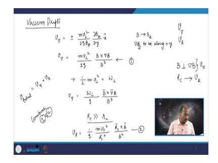
So, in the previous class we have studied the gradient drift and the curvature drift. So, we have also mentioned that the magnetic field imposes a condition that any particle has to always experience both the drifts together; that means, the curvature drift and the gradient drift will always be together.
