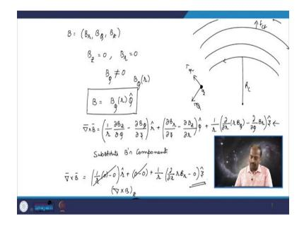
Let us say the magnetic field lines are curved like this. Now, the radius of curvature is this this is R C; now the coordinate system is assumed to be this. So, this is the phi direction the phi cap. So, the magnetic field is directed in the phi cap direction and the centrifugal force is going like this and this direction is the r cap.
