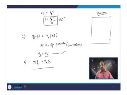
In that cases we will simply write e V which is by the virtue of the potential that is created is equals to k B T; that means, the potential that is existing is roughly of the order of k B T by e.
