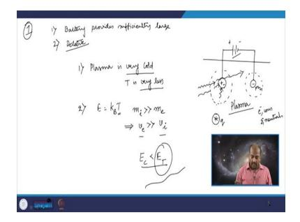
So, let us say we try to put up an electric field inside a plasma, let us say we have a plasma we suspend two electrodes like this and we apply a moderately high potential between these two electrodes. So, what will happen this is the positive terminal this is the negative terminal.
