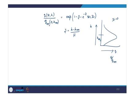
Or we can write the normalized production, the production at any given angle and at any given height with respect to production at 0 angle and the peak production height. As exponential 1 minus z minus e to the power of minus z secant chi.
