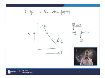
So, we can calculate the time period of these oscillations. So, simply T is equals to 2 pi by lambda, where lambda, is a very important parameter, lambda is called as the Brunt Vaisala frequency. So, this is a characteristic frequency of an atmosphere under a particular condition.
