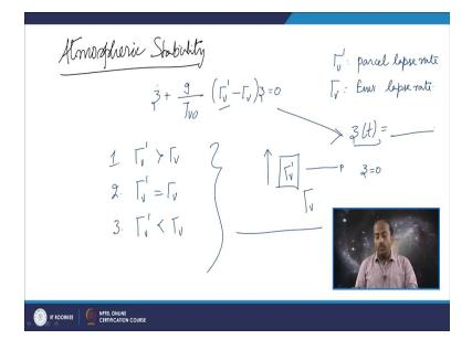
So, we are going to see the mathematical treatment of the various stability conditions; how they will represent the motion of an air parcel in an atmosphere with varying lapse rates between the environment and the parcel, how the atmosphere will allow the parcel to sink or how the atmosphere will allow the parcel to rise further in the atmosphere, right. So, basically the second order differential equation that we have derived in the last class goes something like this.
