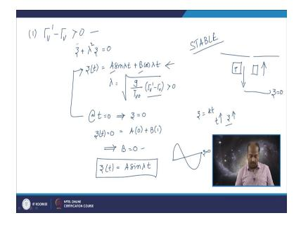
So, let us see, let us take up the first case in which gamma v prime minus gamma v is greater than 0. So, before I do the simple mathematics, let us try to understand what does it mean. So that means that, the lapse rate, the temperature inside the air parcel is decreasing at a faster rate than the environment.
