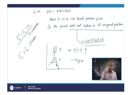
So, let us say at t is equals to infinity, z of t is A in to infinity plus B into 0. So, when time t tends to infinite, the parcels displacement, the parcels position z is also infinite. So, the parcel will not return to its original position. So, when does it happen; if the parcel lapse rate is smaller than the environment lapse rate, then the parcel will be displaced and it will never come back to its original position.
