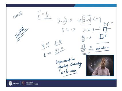
Now, the third case, case III; what will happen if gamma v prime is equal to gamma v? That means, the rate at which temperature is decreasing inside the air parcel is equal to the rate at which temperature is decreasing in the environment.
