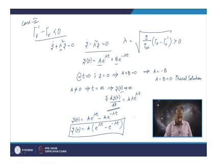
So, this is case II. So, here gamma v prime minus gamma v is less than 0, so that parcel lapse rate is less than the environment lapse rate, right.
