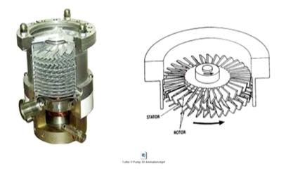
This is the typical picture of a turbo molecular pump and you can see here, there are the stator and the rotor blade which is there and which rotates and ejects the gas molecule. Now the mechanism or the animation of a working principle of a turbo molecular pump is shown in the next video.
