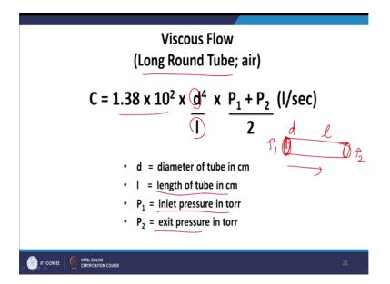
Under the viscous flow, if we consider a long round tube so the conductance is given by 1.38\*10 to the power 2\*d to the power 4/l\*P1+P2/2 liter per second okay. Here d is the diameter of the tube in centimeter, 1 is the length of the tube in centimeter, 1 is the length of the tube, P1 is the inlet pressure and P2 is the exit pressure. So, basically if I have a long round tube like this okay and the diameter here is d and the length is l.
