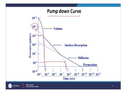
So, this pump down curve is actually a curve of pressure versus time where in y-axis we have plotted pressure in millibar and in x-axis we have plotted time in second. It tells you what is the time scale required to reduce the pressure from a particular value to another certain value. So, whenever we like let us say I have a chamber, so of course it will depend on the volume of the chamber but if the volume of the chamber is standard and if I have a pump.
