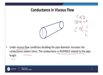
Under viscous flow conditions, doubling the pipe diameter increase the conductance 16 times. Well I mean one important thing to know here that why we are talking about the mean free path, is it only that it is lessen with the pressure. No, actually the mean free path changes whether the flow is viscous flow or a molecular flow but what is the important for that, this viscous flow of the molecular flow is directly related to the conductance and that is we are all interested about.
