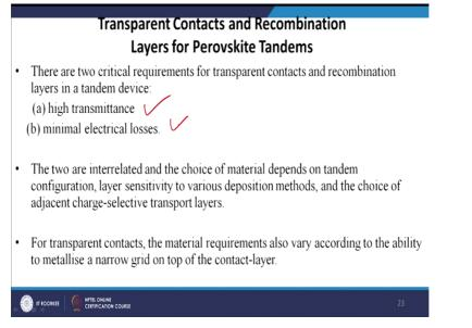
There are lots of research groups which are now working on this area. Now, what about the transparent contacts and the recombination layer for the perovskite tandems because we are talking again and again about this recombination layers and we say that optical and electrical coupling plays a very important role in perovskite devices. Now, there are two critical requirements for transparent contacts and recombination layers in tandem devices.
