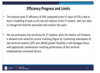
So, the reduced peak 2T efficiency of 39% compared to the four-terminal value of 47% is due to the Kurtz's modeling of the gallium arsenide as the top cell material of the 2T tandem with non-ideal short-circuit or the intrinsic current Jo through the trend for perovskite cells remains the same. So, if I use two-terminal devices, the theoretical maximum efficiency is less than four-terminal devices.
