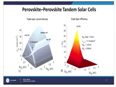
For example, this graph is showing a triple layer current density and here the corresponding triple layer current efficiency is shown here.
