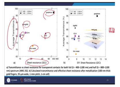
Now, you see that if we look at this graph, so there are so many parameters to optimize. Now, we can use the ITO, we can use graphene layer, we can use thin metal, we can use IZO or we can use the silver nanowires. Now, if we use the different layers, so what the properties is going to change, the transmittance and also the sheet resistance. So, we have to make sure the contact has a very high transmittance over the whole solar spectrum.
