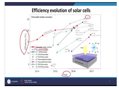
Now, this chart we have also discussed earlier in the beginning of the lecture when we talked about the different generations of the solar cell and here we are showing the efficiency revolutions of the solar cell and as you can see in the y-axis we have the efficiency in percentage and the x-axis is the year.
