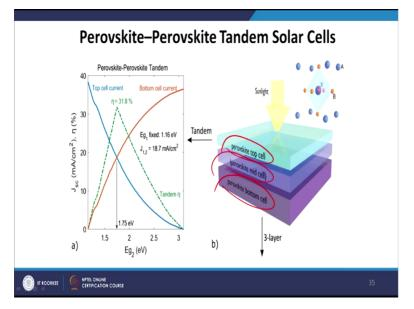
So, here if we take a perovskite- perovskite tandem, you see that the current is changing with the bandgap. So, if we go from 1.5 to a larger bandgap, so the efficiency with the top cell and bottom cell, it is decreasing right. So, it depends on a suitable combination like for example here the perovskite top cells and perovskite bottom cells, so far that was used as a tandem solar cell.
