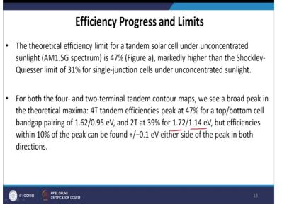
Now, if we look at the efficiency progress and some of the limits of that, the theoretical efficiency limit for a tandem solar cell under unconcentrated sunlight that is AM1.5G spectrum is 47% that is markedly high than the Shockley-Quiesser limit of 31% for a single junction solar cell under unconcentrated sunlight.
