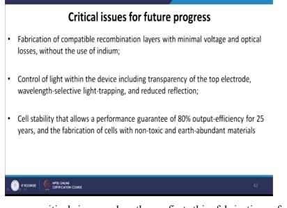
So, there are some critical issues also there, first this fabrication of the compatible recombination layer with minimum voltage loss is one of the problem and we do not need to use the indium in the future. Control of light with the device including the transparency of the top electrode and finally the cell stability that allows a performance guarantee of 80% output for a long period of time at least for 25 years so that it can be compatible with the silicon solar cell efficiency.
