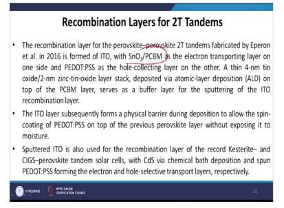
Similarly, the recombination layer for the perovskite-perovskite two-terminal tandems fabricated by another group which use the ITO with SnO2 PCBM as an electron transport
