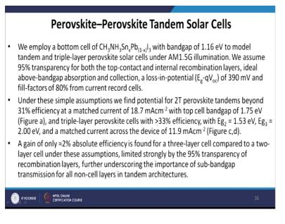
So, we employ a bottom of the CH3NH3 lead iodide with bandgap of 1.16 electron volt to model tandem and triple-layer perovskite solar cells, under this simple assumptions, we found that potential for a 2T perovskite tandem even can reach beyond 30%, 31% efficiency and a gain of only 2% absolute efficiency is found for a three-layer cell compared to a two-layer assumption limited strongly by the 95% transparency of the recombination layer.
