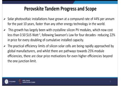
Perovskite tandem progress and scope; solar photovoltaic installations have grown at a compound rate of 44% per annum for the past 10 years, faster than any other energy technology in the world. This growth has largely been with crystalline silicon PV modules, which now cost less than 0.50 US dollar per Watt, following Swanson's Law for four decades reducing 22% in price for every doubling of the cumulative installed capacity.
