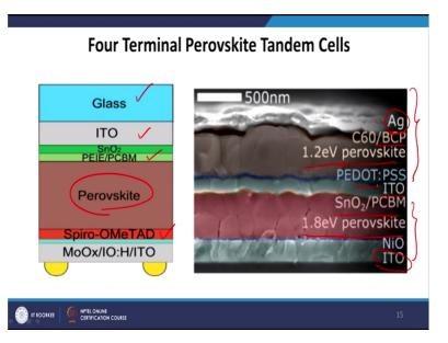
Now, you look at a four-terminal perovskite tandem cells, so here like you know as I said that there is a glass layer and then this is ITO layer okay and then we put the perovskite the active layer between a PCBM layer which acts like an electron acceptor and also a Spiro-OMeTAD layer and finally there is a MoOx coated ITO layer. So, if I take a cross-sectional SEM image, the different layers is showing here.
