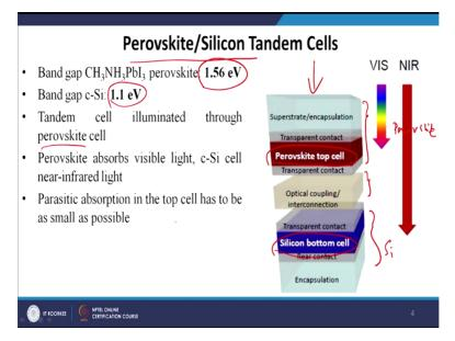
Now, a very common example of the tandem solar cell is a perovskite silicon tandem cells here. As for example, you can look at this device structure here, in the top solar cell we have a perovskite top cell and in the bottom we have a silicon bottom cell. Now, there are two different solar cells, this is a silicon solar cell right and this is a perovskite solar cell and these two solar cells has been connected by an optical coupling.
