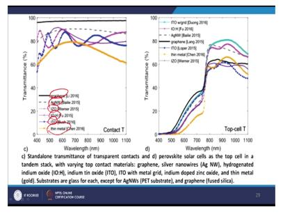
Again, the standalone transmittance of the transparent contacts is shown in the following figure like here the transmittance versus wavelength is showing for a graphene layer, for a silver nanowire, IZO, ITO and thin metal layer. Similarly, the transmittance versus wavelength layer is showing for different types of ITO, AgNW, graphene, ITO and IZO layer.
