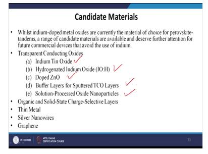
Now, what are the efficient or whatever the ideal candidate materials for making a tandem solar cell. While the indium-doped metal oxides are currently the material of choice for perovskite tandems, a range of candidate materials are available and deserve further attention for further commercial devices that avoid the use of indium. Now, there are several transparent conductive oxide can be used.
