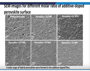
For example, if we use a different, different additives like with the perovskite only perovskite, this is the SEM image if we use 1% TPPI, so the morphology improves. If we use 1% TPPCL, the morphology further changes. So what we mean by changing the morphology is the smoothness, uniformity, crystallinity, and the packing and these all affects the charge transport properties.
