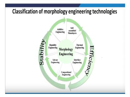
Let us look at this chart, so the classification of the morphology engineering can be many pools. It can be additive engineering, that means while fabricating the active layer we can put an external additive as a solvent. We can use humidity engineering that means if we control the humidity or if we change the humidity that affects the morphology significantly.
