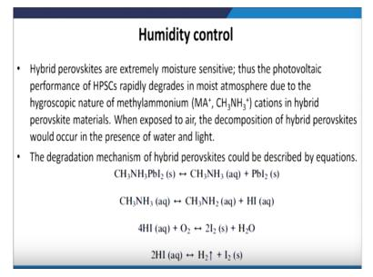
Another very important parameter for making solar cell is the humidity control. Hybrid perovskites are extremely sensitive towards the humidity and they are moisture sensitive thus the photovoltaic performance of the solar cell rapidly degrades in moist environment due to the hygroscopic nature of methylammonium cations in hybrid perovskite materials. There are a series of reactions happens when you expose the CH3NH3 lead iodide to the moisture.
