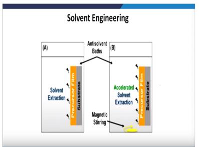
So you can see here the solvent extraction which is happening precursor film in the substrate and yet accelerated solvent extraction is happening due to the magnetic stirring.
