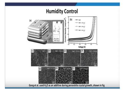
For example, here, you see that on the ITO put PEDOT PSS, perovskite, PCBM, and then BCP and then the silver electrode we have deposited and if we put perovskite and the DFM, the H2O. So as we increase the percentage of the water to 1% to 2% to 5% if we look at I-V curve, the I-V curves falls downs. So the efficiency drops downs and even if you look at the morphology, if we exposed to different, different water vapor, so the crystal started disintegrating.
