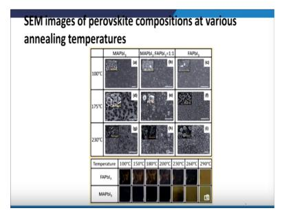
Here we are showing that three different perovskite comparison. For example, MAPbI3 and MAPbI3:FAPbI3=1:1 ratio and for FAPbI3 one is the methyl ammonium and other is the formamidinium and in both case we are using iodine. So if we change the temperature from 100 degree to 175 degree to 230 degrees Celsius, what will happen to the film morphology?
