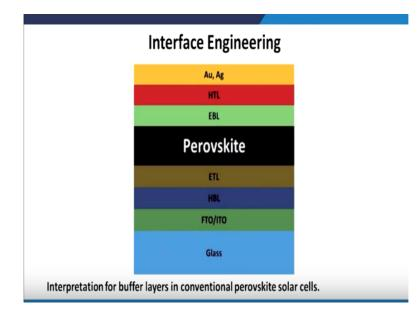
For example, here we are showing the interface engineering. You can see that on the ITO substrate we put a hole blocking layer and an electron transport layer. And then we put a perovskite layer and in the top we have an electron blocking layer and then the hole transport layer.
