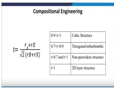
But one has to make sure that the tolerance factor, the value of t, which is basically the radius of the rA + the radius of the X divided by square root of rB + rX that value we need to calculate once we make these changes and if the tolerance factor value is between 0.9 to 1 then it is a cubic structure. If it is between 0.7 to 0.9 then it is a tetragonal or orthorhombic structure. If it is less than 0.7 or greater than 1 then it is a non-perovskite structure.
