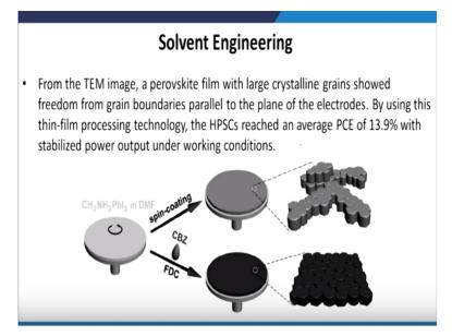
Now you see in this figure, here we have this CH3NH3 lead iodide in DMF solvent which we can spin coat. Now if we spin coat in the presence of that chlorobenzene, so then what will happen. We have in the both the case if we compare the morphology, we get a larger crystallizations, if we use the chlorobenzene as another solvent additive and the efficiency also increase in this case.
