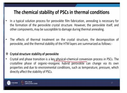
In a typical solution process for perovskite film fabrication annealing is necessary for the formation of perovskite crystal structure. So when we mix the lead iodide and CH3NH3I from a DMF solvent to make a perovskite thin film. So what we do after you allow them to react each other to make a perovskite crystal structure we have to heat them at 120 degrees Celsius and this heating process called the annealing and the annealing gives the desired crystal structure.
