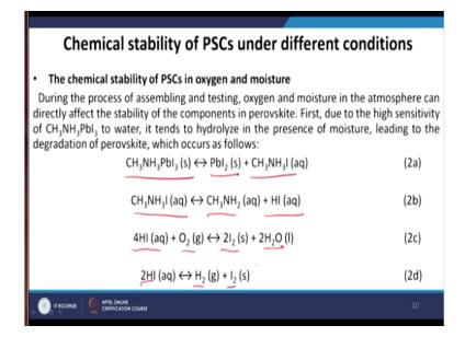
So in this successive reactions we are talking about how the perovskite material undergoes the different kind of disintegration materials. During the process of assembly and testing oxygen and the moisture in the atmosphere can directly affect the stability of the components in perovskite, first due to the high sensitivity of CH3NH3 lead iodide to water it tends to hydrolyze in the presence of moisture.
