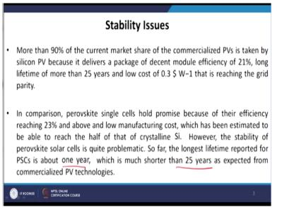
So more than 90% of the current market share of the commercialized PVs is taken by silicon PV. Because it delivers a package of decent module efficiency of 21% long lifetime of more than 25 years and low cost of 0.3 dollar/watt that is reaching the grid parity. So when you use a silicon
