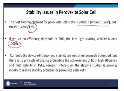
The best lifetime obtained for perovskite solar cell is 10,000 hour around 1 year but the PCE is only about 12%. If we set an efficiency threshold of 20% the best light soaking stability is only 1000 hour. So with a 12% efficiency they can keep 1 year but if we put the target as 20% the lifetime is only 1000 hour. So again that golden triangle cost efficiency and lifetime or stability.
