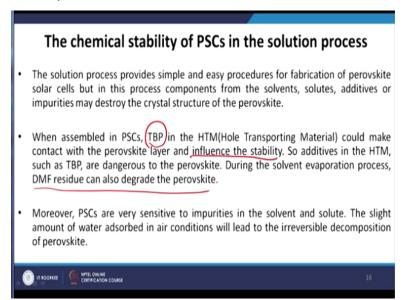
So this is all about interface engineering, now the solution process provides simple and easy procedures for fabrication of perovskite solar cell. But in this process components form the solvents, solutes, additives or impurities may destroy the crystal structure of the perovskite. When assembled in perovskite solar cell tertiary butyl pyridine or TBP in the hole transport material could make contact with the perovskite layer and influence the stability.
