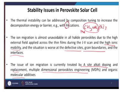
The thermal instability can be addressed by compositional tuning to increase the decomposition energy or barrier as per example with a FA cation. So what does it means like we have seen that when we fabricate the perovskite solar cell what materials we use there we said that every commonly used perovskite material for fabricating solar cell is CH3 NH3 lead iodide. And we say that this organic cation that is also called MA.
