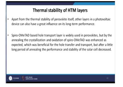
Apart from the thermal stability of perovskite itself other layers in a perovskite photovoltaic device can also have a great influence on the long term performance. Spiro-OMeTAD based hole transport layer is widely used in perovskite but by the annealing the crystallization and oxidation of spiro-OMeTAD was enhanced as expected which was beneficial for the hole transfer and transport. But after a little long period of annealing the performance and stability of the solar cells decreased.
