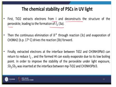
First TiO2 extract electrons from iodine and deconstruct the structure of the perovskite leading to the formations of the iodine. So TiO2 is a very known or good electron extractor, so it extracts the electron from iodine and deconstructs the structure of the perovskite leading to the formation of iodine. Then the continuous elimination of H+ through reaction and evaporation of CH3NH2 drives the forward.
