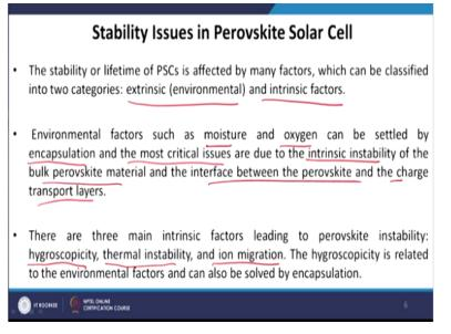
The stability or lifetime of perovskite solar cell is affected by many factors as you mention which can be classified into 2 categories one is extrinsic or environmental like temperature humidity or moisture and another is the intrinsic factors. If the material is such that it undergoes spontaneous disintegration under the sunlight then that is the intrinsic factor. Environmental factors such as moisture and oxygen can be settled by encapsulation that is what we mention that.
