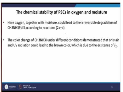
Here oxygen together with the moisture could lead to the irreversible degradation of the CH3NH3 lead iodide according to the reaction 2a and 2d. So we have both oxygen we have both moisture see if I have both moisture and oxygen you see that the CH3NH3I finally disintegrate to hydrogen iodine some CH3NH3I HI all these compound. And sometimes if both are them are present then this reaction is irreversible, this reaction is irreversible degradation.
