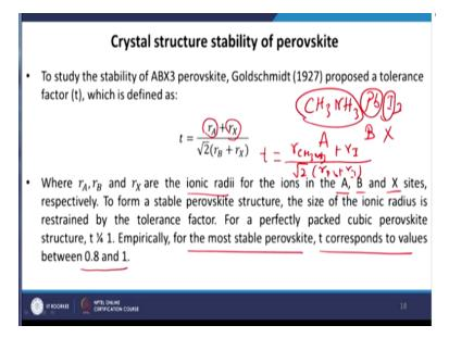
To study the stability of ABX3 perovskite, Goldschmidt proposed a tolerance factor which is defined as we have also talked about this earlier. So tolerance factor is the radius of the A if it thus radius of the X/square root of root 2 rB radius of the B+rx halogen. So in our structure CH3NH3 lead iodine right that was the organic-inorganic halide perovskite. So what is A here this is A, what is B here this is B lead and what is X here, so iodine is the X.
