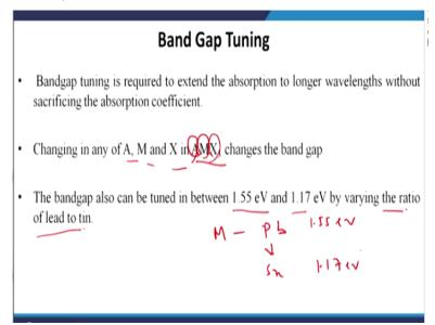
Now as you mention in the beginning one of the advantage of the perovskite material is the band gap tuning. Band gap tuning is required to extend the absorption to longer wavelengths without sacrificing the absorption coefficient. So consider how good it will be, let us say I have a material where the absorption coefficient remains the same even in UV range and visible range
