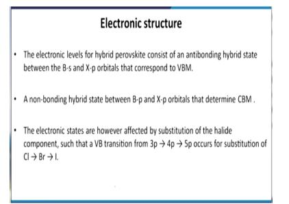
The electronic levels for hybrid perovskite consist of an antibonding hybrid state between the B-s and X-p orbitals that corresponds to VBM. In non-bonding hybrid state between B-p and X-p orbitals then determine the conduction band the electronic states are highly affected by substitution of the halide component such that a VB transition from 3p to 4p to 5p occurs for substitution of chlorine to bromine to iodine.
