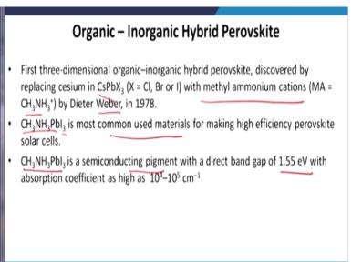
First 3 dimensional organic-inorganic hybrid perovskite discovered by replacing cesium in CsPbX3 with methyl ammonium cations CH3NH3+. So the first example of the organic-inorganic cation and which is still is used very very progressively and commonly is a MA based perovskite structure, where MA or methyl ammonium is CH3NH3+ and it was discovered by Weber in 1978.
