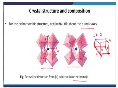
For the orthorhombic structure octahedral tilt about the b and c axis, so if it is an orthorhombic structure then this octahedral this octahedral they tilt around the b and c axis as you can see here. So here this is a perfectly cubic structure but when there is a tilt happens, so you get an orthorhombic structure. And this tilt, if you consider this is as A axis and this as your B axis and the C axis is along the perpendicular to the plane of the paper.
