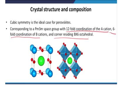
Crystal symmetry is the ideal case of for perovskite corresponding to a Pm3m space group with 12-fold coordination number of the A cation, 6 pole coordination of the B cation and the corner residing BX6 octahedral. We get this cuboctahedral geometry which is shown in this figure. **(Refer Slide Time: 12:47)**
