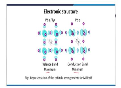
For example here the valence bond maxima the conduction band maxima showing here for the lead where you have s1p orbitals and the Pbp orbitals. Now the orbital arrangements in this 2 case one in the s orbital and this is a p orbital you see that, that is way different in this 2 different geometry. Now as I said that this perovskite material only within a few years of research starting from an efficiency of descent 3.8% is reach today to 22% and that numbers is increasing every day.
