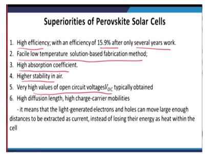
First of all the efficiency is high, it is almost as I said 22% and this number is increasing day by day, with an efficiency of 15.9% only after 5 years of research. Now this data 15.9% is a 2015 data and this is for an indication like starting from 2009 to 2015 or 16 is 4, 5 years of research, efficiency increase from 3.8% to 15.9%. But the today's data is 22% and it is increasing every day, facile low temperature solution based fabrications method.
