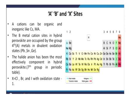
A cations can be organic and inorganic like cesium or CH3NH2 methyl ammonium, the B metal cation sites in hybrid perovskite are occupied by the group fourth metals in divalent oxide states like lead, tin, germanium. The halide anions has been the most effectively component in hybrid perovskite 7 group in perovskite like chlorine, bromine, iodine with oxidation state of 1.
