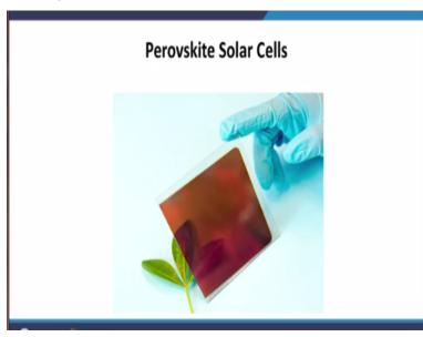
So, the Perovskite solar cell that during the last 10 years it caught the attention of the scientific community as it is efficiency increase all of a sudden from a very desired number to a very high number and this material possess how the properties like tunable band gap, high absorption coefficient. Because of all this excellent photo physical properties, this material is suitable not only for solar cell but also for light emitting diode.
