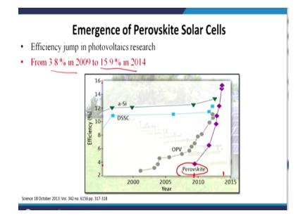
If you look this graph, this figure which is actually a subset of the (()) (01:36) big efficiency graph. So you can see that we are comparing the efficiency verses year for different generations of the solar cell. Now amorphous silicon solar cell the growth is almost constant, dye-sensitize solar cell the efficiency starting from 10 to 11% it remains almost constants and there is a sudden little bit increase here only.
