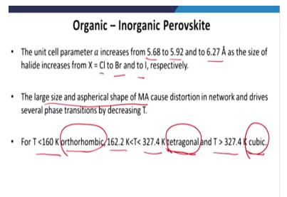
So because of that the intrinsic instability of the device can be enhanced or the intrinsic photo stability of the device can be enhanced. Organic-inorganic perovskite, the unit cell parameter A increase from 5.68 to 5.92 and to 6.27 Armstrong as the size of the halide increase from chlorine, bromine to iodine. If you change from chlorine to bromine to iodine, so what happens the unit cell parameters change from 5.68 to 5.92 to 6.27 Armstrong.
