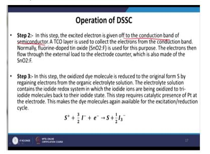
Then the second step is that the excited electron is given to the conduction band of the semiconductor. So it is given off to the conduction band of the semiconductor, what is the semiconductor here TiO2. Now a TCO layer or a transparent conductive oxide layer, so TCO stands for transparent conductive oxide. So for example ITO or FTO is a transparent conductive oxide, so light can pass through them that is why they are transparent.
