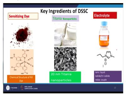
Here we are showing certain kind of dyes like one of the very popular dye which is used in the DSSC device is N3 dye and it has a structure like this where the ruthenium molecule is in the center and it forms a very giant complex which is surrounded by some benzene ring and some
