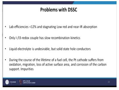
So there are some application, good application also do the DSSC but there are also some problems. As I said that the efficiency even after doing 20 years of research is still less than 20% whether in perovskite solar cell it has reach to 20 to 23 % efficiency or in single crystal or in amorphous even solar cell we can get routinely 12 to 15% efficiency. And this is due to the low absorptions in the near IR region.
