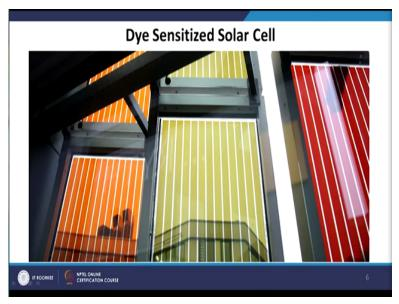
Here in this picture we are showing there are some transparent window of even transparent door which was fabricated by this dye sensitized solar cells. Now one of the biggest advantage that we already mention previously that this organic photovoltaics including this dye sensitized solar cells they can be make flexible as well as transparent. So that means we can put it on any substrate on which we like to put it and at the same time light can also transmit through them.
