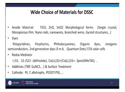
Single crystal mesoporous film nano dots, nanowires, branched wires or gyroid structure, people have used different kind of structures. And this role of the structures is also manifold some of them actually help to confine the electric field, some of them actually helps to increase the internal electric field and to increase the output current in the devices. Now as a dye we have a choice of using different kind of polymers or different kind of small molecule.
