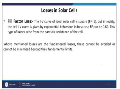
Fill factor loss, the IV curve of the ideal solar cell is square fill factor is 1 but in reality the cell IV curve is given by an exponential behavior. In best case FF can be 0.89 this type of loss arises from the parasitic resistance of the cell. As I said that if I have a higher values of the series resistance and a lower values of the shunt resistance then fill factor changes. And looking at the fill factor we can say how good is this devices.
