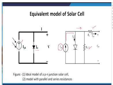
Here we are showing the equivalent model of a solar cell as you can see the first diagram the equation the figure1 is the ideal model of a pn junction solar cell. Here we have a current source Iph is this one which is connected in parallel with a diode. And then since this is an ideal model,
