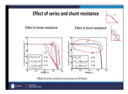
Now what will happen if the series resistance changes and if the shunt resistance changes, so that will directly affect the IV curve. As you can see here the IV characteristics like the fill factor value is showing for series resistance value 0, when the series resistance value is 0 then you see that this curve is this blue curve this one. When the series resistance is 10 ohm centimeter square then this portion of the curve is changing.
