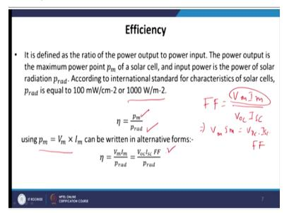
So as we said like efficiency it is defined as the ratio of the power to power input like all engines they provide some kind of power output when you put some power input. Solar cell also take this power input from the solar radiation and it what it does like you know it converts the light energy to the electrical energy. And this electrical energy is nothing but comes in a terms of the current and voltage and this product of current and voltage we call it as a power.
