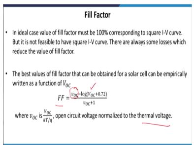
It is also worthwhile to mention that like the fill factor value can tell you how good the quality of the solar cell. In ideal case the value of fill factor must be 100% that means there should not be any deviation from the square nature. But in real solar cell there can be deviation and where this deviation is coming from due to the resistance, what kind of resistance, it can be series resistance or it can be shunt resistance what contribute to the resistance.
