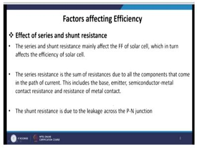
Now because of the series resistance and sun resistance fill factor value can change significantly. Now the series and shunt resistance mainly affect the fill factor of the solar cell which in turn affects the efficiency of a solar cell. The series resistance is the sum of the resistance due to all components that come in the path of the current. So whenever current flows in a circuit whatever the source of resistance it fills while going to the electrode that is acts as a series resistant.
