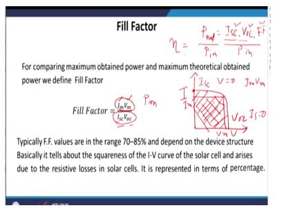
By definition fill factor is the maximum power that is the Im times Vm the maximum current times the maximum voltage/maximum theoretical power which we get from the circuit that is short circuit current and open circuit voltage. So ImVm that is the maximum obtained power from the device which is like you know the maximum power which we can get from the device, if the device is an ideal solar cell.
