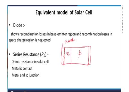
So series resistance is a ohmic resistance in a solar cell it is comes due to the metallic contact or more precisely metal and semiconductor. Let us consider this is our solar cell where the n side is narrow and heavily doped, so that the depression regions extent inside the p regions, to compute a solar cell we put a metallic contact on the front end and ohmic back contact at the back end. Now this metallic contact made as schottky kind of barrier at this metal semiconductor interface.
