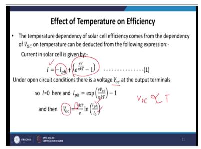
Now temperature also plays a very important role in measuring a efficiency of a solar cell. For example the temperature dependency of solar cell it comes due to the changes in the Voc as you change the temperature. And we can reduce an expression for that, so as you know that current in a solar cell that can be retain as **as** a combination of 2 part, one is the photocurrent minus Iph and another is the diode current, I0 e to the power ev/eta kT - 1.
