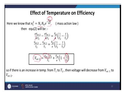
We know that ni square is Nc times Nv \* e to the power -Eg/kT law of mass action if we remember where Eg is the band gap and T is the temperature. So then eVoc2/kT2 - eVoc1/kT1 = Eg/k 1/T2 - 1/T1 or if we take k as a common from here this k and this k and this k cancels out giving you Voc2/T2-Voc1/T1 = Eg/e so this e we are taking out in the right hand side into 1 over T2 - 1 over T1 or you get Voc2=Voc1T2/T1 + Eg/e 1 - T2/T10k.
