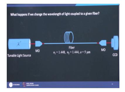
So, what I do? I take a fiber which is given which is fixed. So, n 1 n 2 and a they are fixed, now I launch light into this fiber monochromatic light from tunable light source tunable laser whose wavelength I can change, and I capture the output from the fiber using a microscope objective and image it onto a CCD. So, that I can see the pattern what I wish to do is when I change the wavelength I would like to see how the output pattern changes.
