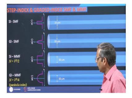
Now, you can also have a step index and graded index fibers, this is step index single mode fiber where the core diameter is about 10 micron and the refractive index in the core and in the cladding is uniform. In the same dimensions you can also have refractive index in the core which changes with radial position, then it is called graded index single mode fiber.
