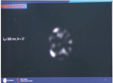
I further change it to 300 nanometer the number of modes are now 17, I increase it to 350 nanometer number of modes are 13, 400 nanometer number of modes are 10.
