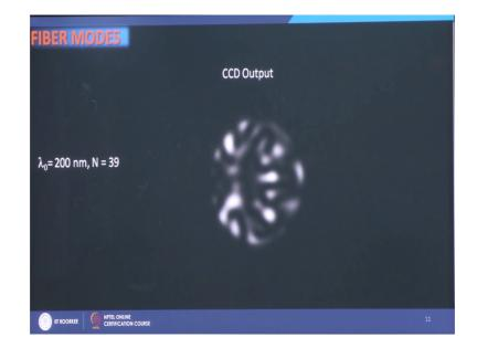
Let me perform this let me see the CCD output, when I launch wavelength 200 nanometer light of wavelength 200 nanometer, then this is the kind of pattern I see. I see a speckle pattern this is nothing, but the interference between all the possible modes of
