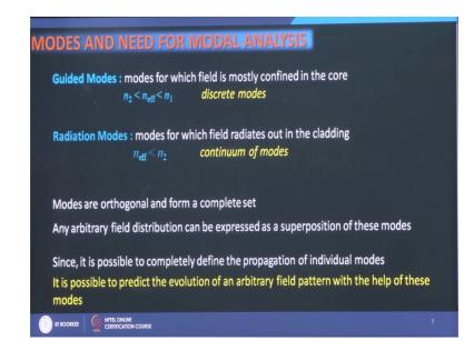
So, in a fiber these kind of intensity patterns I have seen that they extent to cladding, but energy does not propagate out up to infinity into cladding. The energies still guided in the core, it certain part of the energy is only extended to the cladding and these modes are called guided modes of the fiber, and for these modes n effective lies between n 2 and n 1, and there are only certain discrete patterns certain discrete field patterns. So, these are discrete modes.
