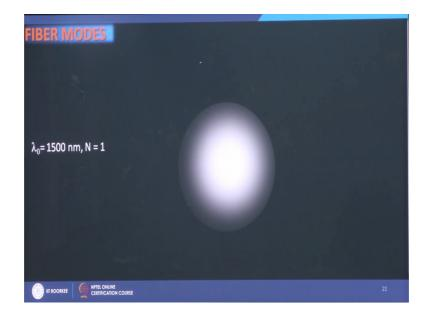
And you just see the pattern here 1200 nanometers again 2 modes and when I have 1500 nanometer I see a very clean pattern here, which is the fundamental mode which means that there are no speckles here which means that there is only one mode.
