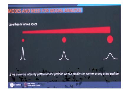
Let us first understand modes for that let me first take a laser beam a typical beam from a laser pointer for example, or typical beam from a single mode helium neon laser. If I look at this beam here when it just exits from the laser this spot looks like this, if I capture this beam just at the exit of this laser as soon as it comes out then this spot looks like this. And if I see how the intensity of this spot varies along a diameter it looks like this.
