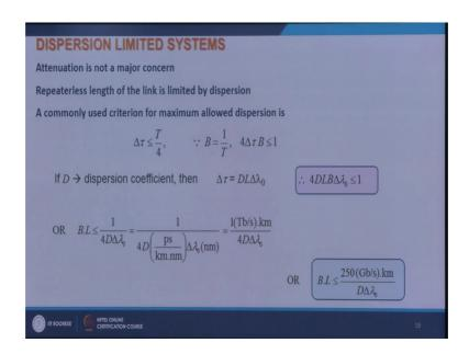
And a commonly used criterion for maximum allowed dispersion is that the broadening should be less than or equal to T by 4 where T is the bit slot or bit duration and since B is equal to 1 over T. So, I can write this as 4 times delta tau times B is less than or equal to 1.
