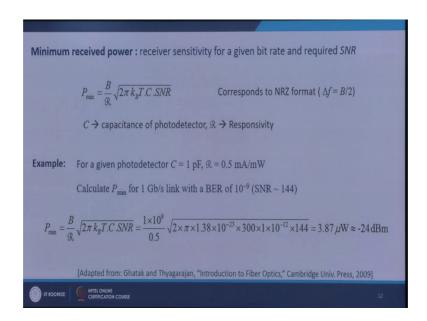
So, what is the sensitivity of a detector for a given bit rate and SNR so that I can distinguish my one from 0 very well. It is given in terms of minimum received power what should be the minimum power that a receiver should receive, and it is given by b divided by responsivity bit rate divided by responsivity times two square root of 2 pi k B T times C times SNR.
