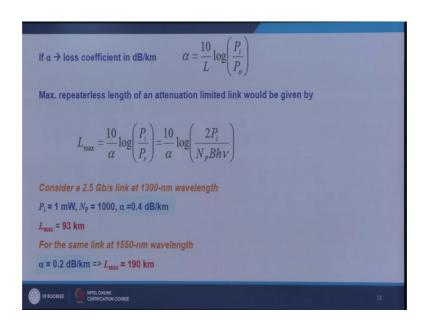
Now, if alpha is the loss coefficient d B per kilometer, then alpha is equal to ten divided by L log P i over P out and. So, the L max is equal to 10 divided by alpha log P i divided by P r which is minimum average received power, and if I put the expression for that from previous slide it comes out to be like this.
