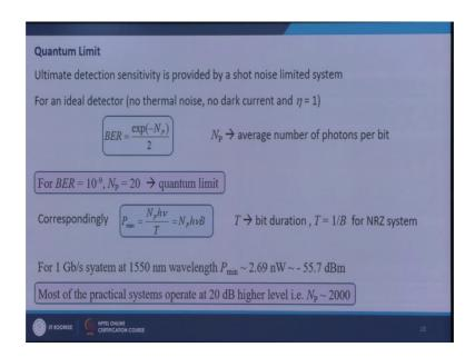
Where N p is the average number of photons per bit for BER is equal to 10 to the power minus 9, if you put it here then N p will come out to be about 20. So, this is the quantum limit and corresponds to the ultimate detection sensitivity.
