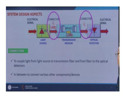
Then we have connectors at several places took up a light from light source to transmission fiber and from fiber to the optical detector, and in between also we put several optical fiber based components. So, we will require connectors. So, these connectors will cause some loss each connector will have certain loss. So, we will have to take into account that.
