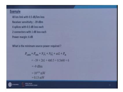
Let me have a forty kilometer link with 0.5 d B kilometer 0.5 d B per kilometer loss receiver sensitivity is minus 39 d B m.
