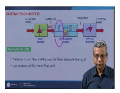
So, whatever fiber we are using we will have to take into account the loss of that fiber at the operating wavelength. So, this loss depends upon the fiber used and of course, the wavelength of operation.
