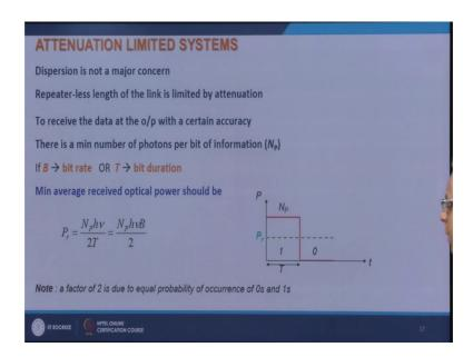
So, how do I get this? Well to receive data at the output end with certain accuracy, I need to have minimum number of photons per bit information and if B is the bit rate and T is the bit duration, then the minimum average received optical power should be N p h nu divided by 2 T which is N p h nu B divided by 2.
