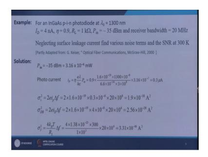
So, I take an example of indium gallium arsenide P i n photo diode at lambda naught is equal to 1300 nanometer, which has I D is equal to 4 nano amperes, quantum efficiency 90 percent, load resistor is 1 kilo om and P n is minus 35 d B m and receiver bandwidth is 20 megahertz. So, I would like to find out various noise terms and SNR at 300 k neglecting the surface leakage current.
