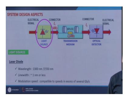
So, what we have the overall system that we have electric signal, which comes out from data, data is in the form of electric signal which drives light source generates optical pulses, then this optical energy is coupled to transmission medium which is optical fiber using connector, then in between we can have several optical fibers.
