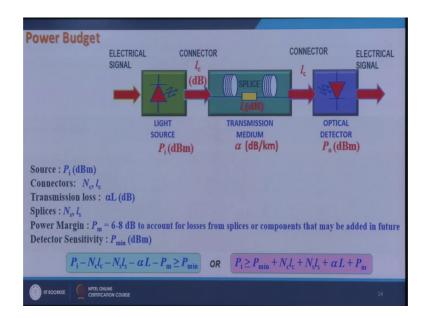
So, as we have seen that we have the light source then we have connector splices loss due to transmission medium, then sensitivity of the detectors and so on. So, how much power my light source should have or what should be the sensitivity of the detector if I take into account all the losses.
