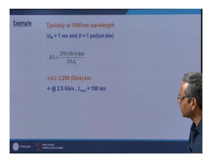
So, if I have a system with b is equal to 1 picoseconds per kilometer nanometer at 1300 nanometer wavelength with delta lambda naught is equal to 1 nanometer which is the typical system at 1300 nanometer wavelength you have very small dispersion.
