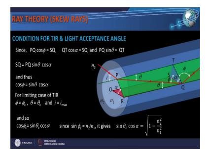
It is incident it hits the point Q at core cladding interface and then it is reflected. Let me make this plane consider this plane which contains this incident light and reflected light which is represented by green here, and this is the normal QT is the normal at the core cladding interface and then let me also consider another plane which is a longitudinal plane, but which contains this line this longitudinal line which passes through Q.
