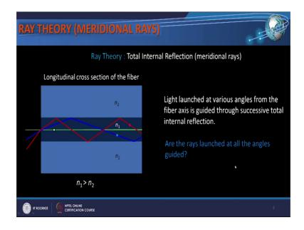
Now, let us look at light guidance by meridional rays. So, if I launch light at various angles into this fiber this is a longitudinal cross section of the fiber, then what happens is that the rays launched at different angles will be guided through successive total internal reflections. Now the question is are the rays launched at all the angles guided or there are only certain range of angles that would be guided.
