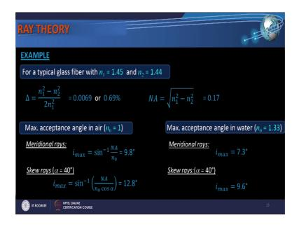
The maximum acceptance angle in air is can now be given by for meridional rays as imax is equal to sin inverse n a over n 0, which is about 10 degrees 9.8 degrees and for skew rays for alpha is equal to 40 degrees it is about 12.8 degrees. If I put the same fiber in water where the refractive index is 1.33, then for meridian rays imax becomes 7.3 and for skew rays it is 9.6.
