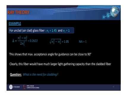
If I consider an unclad fiber than n 1 is equal to 1.45 and n 2 is one which is basically air then delta is 0.26 and square root of n 1 is square minus n 2 square minus is equal to 1.05 which means n a should be equal to 1. This shows that the maximum acceptance angle for guidance can be close to 90 degrees because n a is equal to 1 sin imax is equal to 1 clearly this fiber would have much more light gathering capacity as compared to cladded fiber.
