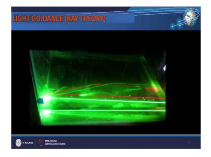
This is one very simple experiment that you can do you can fill a transparent tank with water and then you send the laser beam at different angles, and you find that if the angle of incidence is larger than the critical angle there is total internal reflection at the interface of water and air.
