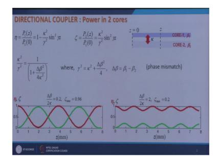
Then the fractional power that is in core 1 is given by 1 minus kappa square over gamma square sin square gamma z. And the fractional power in the core 2 is given by kappa square over gamma square sin square gamma z, where gamma square is equal to kappa square plus delta beta square by 4 and delta beta is nothing but the phase mismatch which is the difference between the propagation constants, beta 1 and beta 2.
