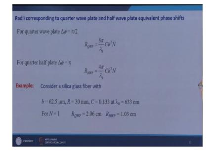
In bulk optics if I have birefringent crystals then out of these crystals I can make quarter wave plate half wave plate. Quarter wave plate means apart difference of lambda by 4 or phase shift of pi by 2.
