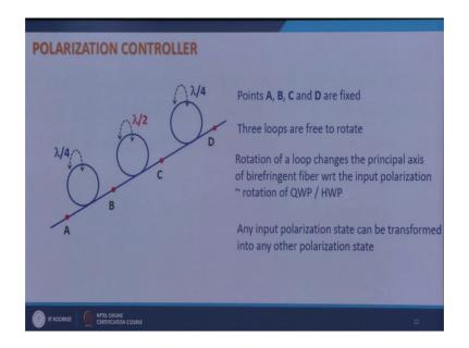
So, with the help of this with the combination of these loops: I can virtually obtain any polarization state, how? Well, I take a fiber and make loops like this. Let us say the radius of the loops are such that or radii of the loops are such that this loop introduces a part difference of lambda by 4. So, this is the quarter wave plate this is equivalent to half wave half wave plate and this is again quarter wave plate.
