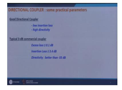
For a typical 3 dB commercial coupler excess loss is less than or equal to 0.1 dB. Insertion loss says about 3.4 dB or less and directivity is better than minus 55 db.
