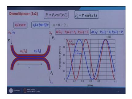
So, if we send 2 wavelengths lambda 1 and lambda 2, through this device then what will happen. Let us say at lambda 1 the coupling coefficient is kappa 1, and at wavelength lambda 2 the coupling coefficient is kappa 2. We know that for phase matched case let us consider phase matched case for convenience P 1 is equal to P I cosine square kappa L this is the power in core 1, and P 2 is P I sin square kappa L power in core 2.
