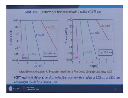
Here I have plotted the loss of 100 turns of a fiber, quite with the radius of 3.75 centimeter and this loss I have plotted as a function of core radius, for different values of core cladding index difference relative index difference, and in this figure I have plotted it at wave length 1300 nanometer.
