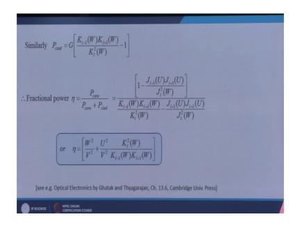
So, I have the fractional power in the core given by this expression. Now I am interested in how does this look like when I vary V, when I vary the parameters of the fiber and in this way I vary the value of V normalized frequency, then how the power in the core and the cladding is distributed how this distribution changes. So, for that let me plot this eta frictional power as a function of V and this has been taken from this paper. I have adopted this. So, it is slightly modified.
