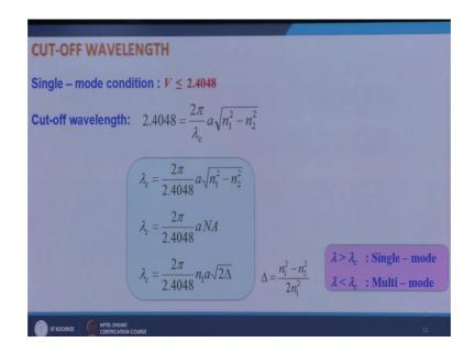
If you look at a fiber, then the single mode condition is given by V is less than equal to 2.4048 equal to sin corresponds to the limiting case, and V is given by V is given by 2 pi over lambda naught times a times square root of n 1 square minus n 2 square.
