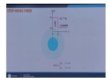
So, again we are analyzing this kind of step index optical fiber, and we know that the power is proportional to if psi is the modal field which is basically the electric field, then the power is proportional to the electric field square integrated over the entire transverse cross section.
