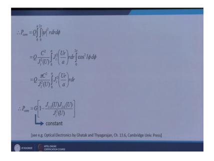
So, P core is this and if I now substitute the modal field of the core, then it would be of the form J l square U r over a r d r and then phi. So, phi part would be cosine square l phi t phi, and this would be the constant which comes out.
