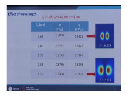
I have tabulated the fractional power in the core for LP 01 which is the fundamental mode and LP 11 which is the first higher order mode. So, I see that at 0.65 micrometer wave length, 90 more than 98 percent power for LP 01 mode is located in the core and 96 percent power is located in the core for LP 11 mode. So, as I increase the wave length I see the general trend that the power in the core for a given mode decreases.
