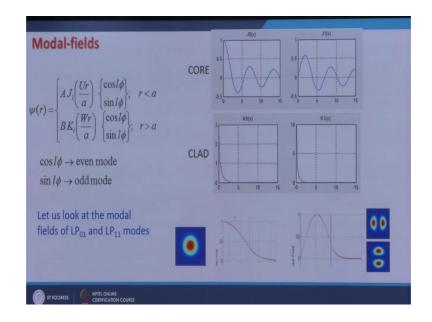
Now, let us look at how the modal fields look like. So, the total modal field would be given by the radial part and the angular part or Azimuthal part. In phi direction I can have solutions cosine L phi and sin L 5 and I label these 2 solutions by 2 different names I call cosine alpha solution as even mode and sin alpha solution as odd mode.
