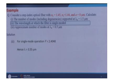
Second is the wave length at which the fiber is single moded, if I want to find out the wave length at which the fiber is single moded or the wave length range in which the fiber is single moded then I know the single mode condition for a fiber is V should be less than 2.4048 and I have the expression for V.
