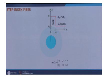
So, this is the step index fiber which we are analyzing, which has a high index core of refractive index n 1 of radius a and the cladding of refractive index n 2.
