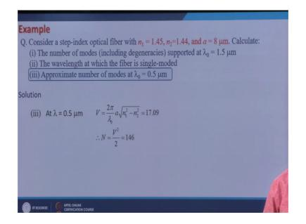
Third part is approximate number of modes at lambda naught is equal to 0.5 micrometer. So, I again calculate the value of V at 0.5 micrometer, and it comes out to be about 17 which is much larger than one, then I can find out the approximate number of modes by V square by 2 and it comes out to be about 146. So, this fiber will support 146 modes.
