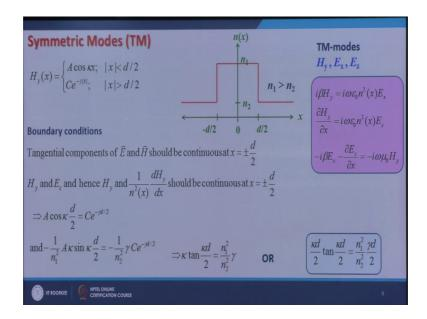
In this case also I can make use of the symmetry of the problem and divide these solutions into symmetric and antisymmetric. So, for symmetric modes my H y would be a cosine kappa x in the guiding film, and Ce to the power minus gamma mode x for
