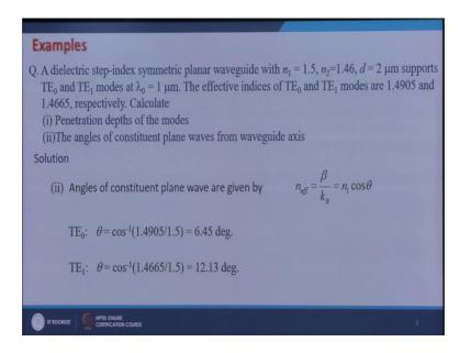
So, for TE 0 mode this theta would be cos inverse n effective over n 1. So, it would be 6.45 degrees and for TE 1 it would be 12.13 degrees. So, TE 0 mode is nothing but is nothing but the superposition of 2 plane waves, making angles making angles plus minus 6.45 degrees from the waveguide axis. And TE 1 mode is the super position of 2 plane waves which make angles plus minus 12.13 degrees from the waveguide axis.
