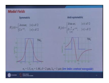
So, the slope is not continuous. Although here I see that the slope is also continuous at the boundary, but the, but rigorously it is not continuous. It is the discontinuity in the slope is. So, small that it does not show up because if you look at n 1 and n 2 n 1 and n 2 are very close. So, if it is weakly guiding if the waveguide is weekly guiding the n 1 the values of n 1 and n 2 are very close to each other than that would not show up here.
