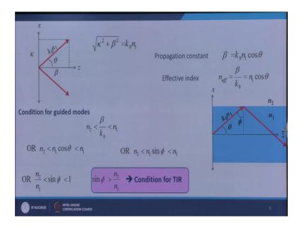
And what happens is if I do this kappa square plus beta square it comes out to be k naught n 1 and k naught, n 1 is nothing but the propagation constant with which a plane wave propagates in an infinitely extended medium of refractive index n 1.
