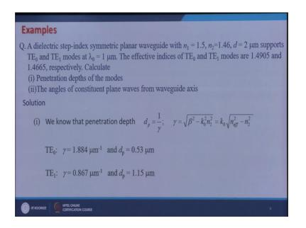
And it supports 2 modes TE 0 and TE 1 mode at lambda is equal to 1 micrometer. And if I find out the effective indices of these 2 modes they come out to be 1.4905 and 1.4665 respectively.
