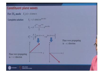
So, it is given in the core or in the guiding film it is given by E y of x is equal to a cosine kappa x. If I write down the complete solution that is the z part and t part also, then it would be a cosine kappa x E to the power i omega t minus beta z.
