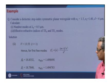
So, the number of modes supported would be 9 I can see this value of V is very large. So, it would be now easier for me to find out the propagation constants of TE 0 and TE 1 mode, even without solving the transcendental equation.
