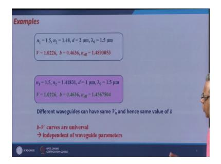
If I calculate the value of V from here it comes out to be 1.0226. I go back to those b V curves and read the value of b from here corresponding to this value of V it comes out to be 0.4636. And then I find out the value of an effective, which comes out to be 1.4893053 ok.
