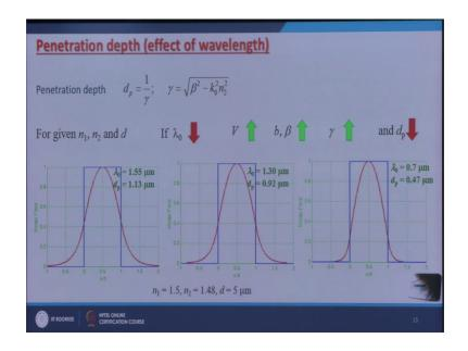
If I am increasing the value of b that is beta square minus k naught square n 2 square increases gamma increases. So, penetration depth decreases. So, this is the field of a given waveguide when operated at 1.55 micrometer you can see how much the field extends outside and when I decrease the wavelength to 1.3 the field is pushed more towards n 1 region and when it is 0.7 micrometer than the penetration depth is much smaller.
