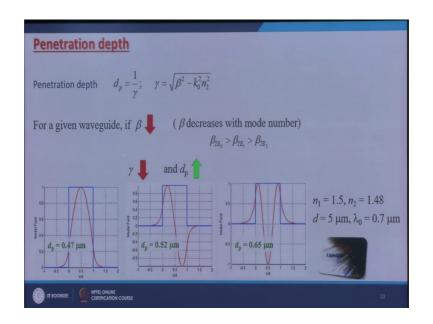
I can see the effect of this penetration depth I can see this penetration depth. So, for a given waveguide if beta decreases because penetration depth is defined by 1 over gamma and gamma is equal to beta square minus k naught square n 2 square it is a square root.
