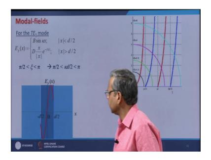
Now for TE 1 mode, psi would lie between pi by 2 and pi psi would lie between pi by 2 and pi, because this the green curve will cut the blue curve only in this region. Now if I which means that kappa d by 2 would lie between pi by 2 and pi, and now in the same way if I plot the field in the guiding film first. So, there would be a sin function ok.
