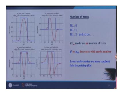
And if I go on then TE 2 mode has 2 0 crossings TE 3 mode has 3 0 crossings which means that if it is TE m mode then it will have m number of 0s ok. It will have m 0 crossings, this is one thing another thing that I see is when I solve this, that with the number of modes the propagation constant decreases right, if you remember the b V curves.
