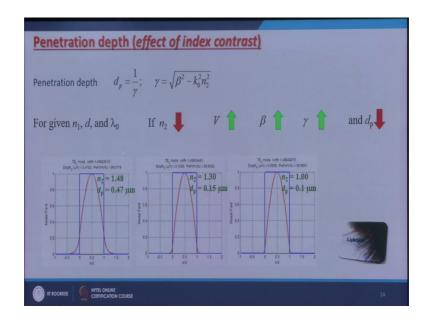
What is the effect of index contrast on penetration depth? Well again, the penetration depth is given by this, so for a given n 1 d and lambda naught. Now if I change the value of n 2 and hence the index contrast, for example, if I decrease n 2 if I decrease n 2 then the value of V increases. The value of V increases because n 1 square minus n 2 square increases. If V increases the propagation constant if V increases the propagation constant increases and penetration depth decreases.
