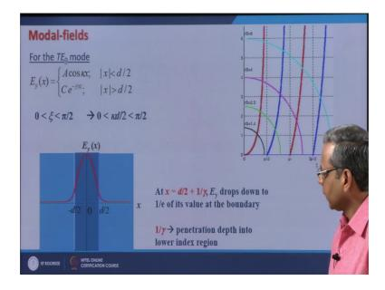
So, the modal field will be given by E y of x is equal to A cosine kappa x in the region mode x less than d by 2, and Ce to the power minus gamma mode x for mode x greater
