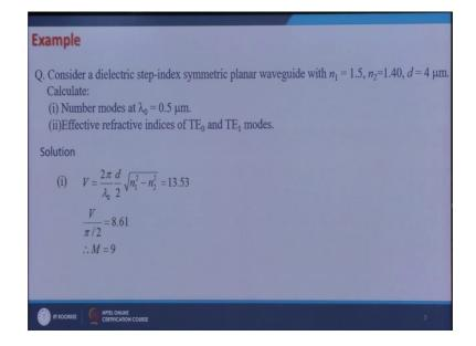
I consider a step index planar symmetric waveguide with n 1 is equal to 1.5, n 2 is equal to 1.4 and d is equal to 4 micro meter. And let us calculate the number of modes at 0.5 micro meter and effective refractive indices or effective index of modes of TE 0 and TE 1 modes.
