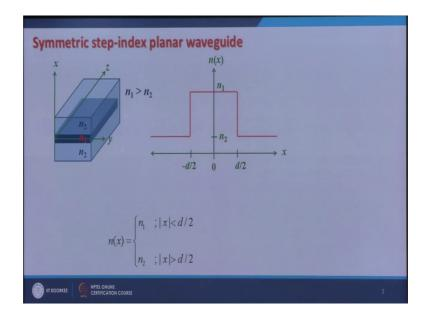
So, what we did we categorize the modes of this waveguide using the symmetry of the structure into symmetric and antisymmetric modes and for symmetric modes.
