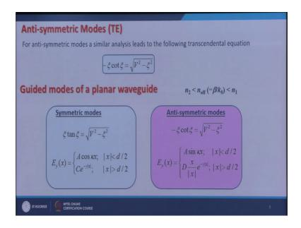
So, the guided modes of a planar waveguide where a symmetric or antisymmetric there it fall in the in the range of an effective line from n 2 to n 1, and they are given by E y of x is equal to A cosine kappa x for mod x less than d by 2 and C e to the power minus gamma x for mod x greater than d by 2 for symmetric modes this is the symmetric solution. And the values of beta which are allowed are given by psi tan psi is equal to square root of V square minus psi square.
