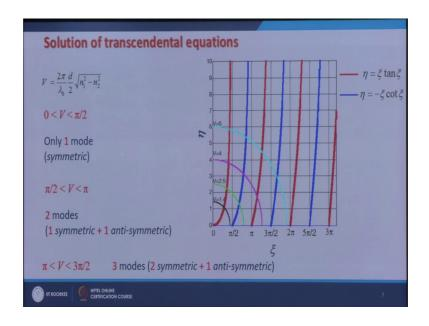
So, let us plot these. So, here the red line, the red line shows the equation eta is equal to psi tan psi, which corresponds to symmetric modes. And these blue lines they show the plot for eta is equal to minus psi cot psi they correspond to antisymmetric modes. And these circles for different values of V are basically psi square plus eta square is equal to V square.
