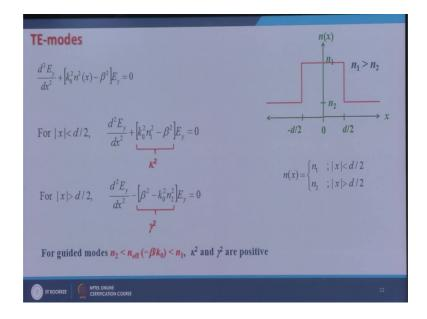
So, this is the wave equation for TE-modes and this is the n x. So, how do I solve it? Well I find that in this region and in this region and in this region in all the 3 regions the refractive index is constant although when I go from here to here and here to here I encounter index discontinuity, but on this side and on that side the refractive index remains constant.
