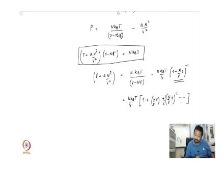
So, that the equation of state becomes a N square over V square times V minus N sigma sorry not b this is going to be sigma and sigma is going to be NK B T. So, you nicely come up with the Van der Waals equation of state right.
