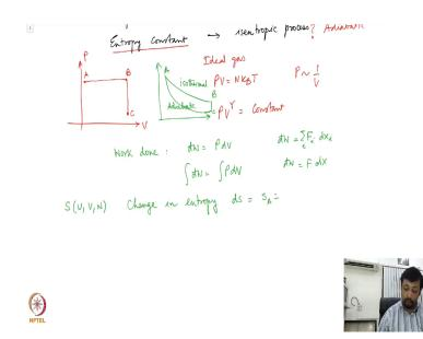
The work done for this particular system is P d V. In general is F i d X i sum over i. If you have one force then it is just F 1 sorry if you have just one thermodynamic coordinate; for example, here I have only one extensive coordinate for the hydrostatic system which is the volume because n is typically (Refer Time: 36:32) then this is the case is the work done.
