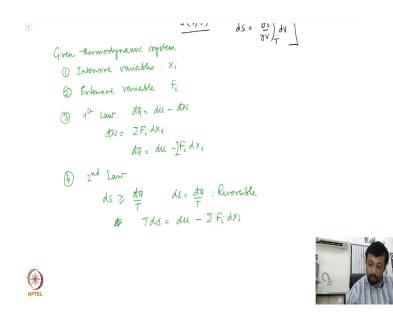
Again, let us just very quickly summarize that for a given thermodynamic system I have a set of intensive variables and a set of extensive variables. X i F i 1st law is delta Q or we will write it down in the differential form d cut Q is d u minus d cut W; d cut W is F i d X i so, that d cut Q is equal to d u minus F i d X i.
