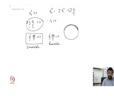
Therefore, it follows that Q T 0 must be less than 0, but what is Q T 0? Q T 0 is sum over Q i 0 which is sum over t 0 Q i over T i this implies that Q i T i sum over I must be less than equal to 0.
