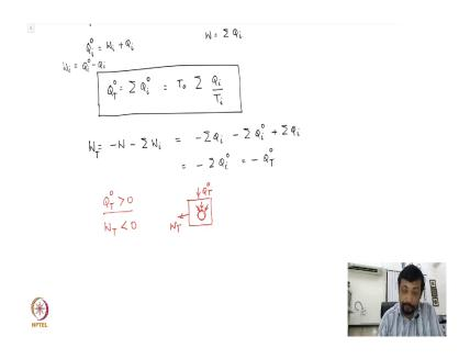
The total work done is minus W plus we will put a subscript because work is the energy which is flowing out of the system therefore, in our convention it should be minus W i. So, minus W is minus sum over Q i and then we will write down this as minus sum over Q i 0 plus sum over Q i this follows from here where I can recast this equation as W i is Q i 0 minus Q i.
