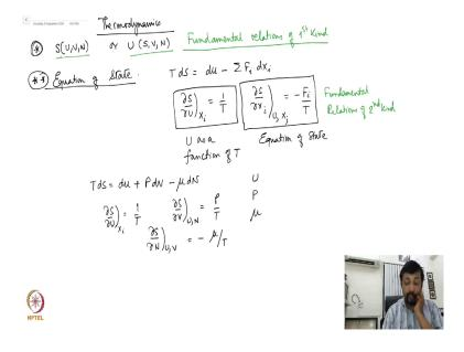
Since, I have already written down the 1st law. So, del S del V is e U constant and N constant is P by T and del S del N U constant and V constant is minus mu by T. So, you can replace this over here and integrate out to determine S as a function of U, V and N right.
