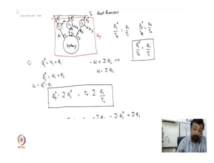
So, imagine that I have a system that works in a cycle. So, we will call this cycle as p and this is my system and this system receives an amount of heat Q 1 at temperature T 1 it receives amount of heat Q 2 at temperature T 2 and then again let us say it does it with Q 3 it receives an amount of heat Q 3 at temperature T 3 and so on and so forth.
