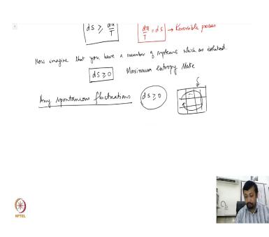
Of course, this also has to mean that the system is isolated system right. So, your joint equilibrium or the final thermodynamic state is the one which has the maximum entropy. So, any spontaneous fluctuation; why do we say a talk about any spontaneous fluctuations? Because your system which is made up of smaller subsystem is insulated from the outer world. So, therefore, there is no heat that no energy which flows out.
