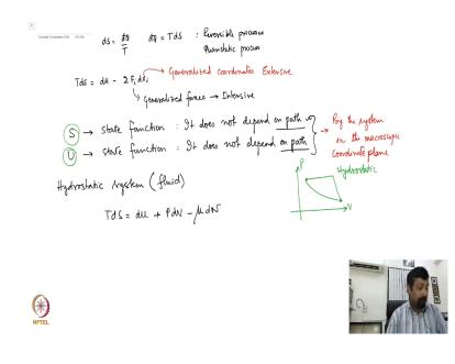
So, I know that d S is d cut Q by T. So, in principle therefore, it follows that d cut Q by d S and this is true for all reversible processes or quasi static processes which are necessarily reversible. So, therefore, I can write down rewrite down my 1st law as T d S is equal to d u minus sum over F i d X i.
