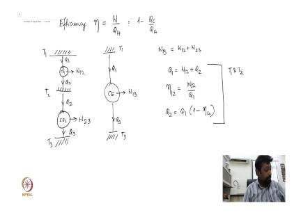
So, question now remains is what should be the efficiency eta, which is W over QH which is 1 minus QC over QH. Now for this case we will consider 2 Carnot engines one at T1. So, operating the second one T2 and yet a third one which is at T3. So, it takes an amount of heat Q1 dumps it to Q2 does an amount of work W 1 2 this one takes an amount of work Q2 as amount of heat the same amount of heat Q2 and does an work W 13 and dumps an amount of heat Q3.
