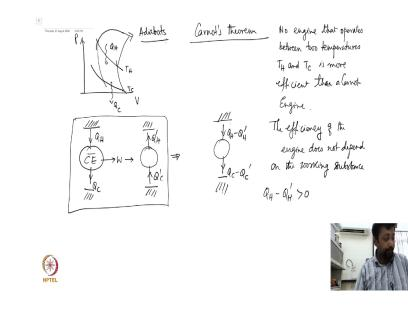
So, if I want to look at the PV diagram then I have the isotherms and I have the adiabats right. So, the isotherms is where the heat is taken this is TH and this is TC and the adiabat is and the second one is where the heat is dumped the isotherm corresponding to TC. These 2 are adiabats and therefore there is no heat exchange that is allowed. So, this is the simplest form of a Carnot engine.
