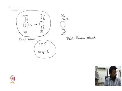
So, if I let us violate Kelvin's I mean by purpose so I have a machine with which I denote by bar, because again it is violating a statement it draws an amount of heat Q from the hot reservoir and does an amount of heat W completely converting this heat into W.
