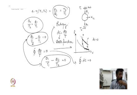
So, if I now write down one minus eta T1 comma T2 as Q 2 over Q 1 and this we saw was T2 over T1. Interestingly let us just look at this part of the equation and recast it in the following way. Now when you look at the Carnot engine which operates by taking an amount of heat Q 2 sorry an amount of heat Q 1 from the hot reservoir dumps an amount of heat Q 2 the cold reservoir does an work W 1 2.
