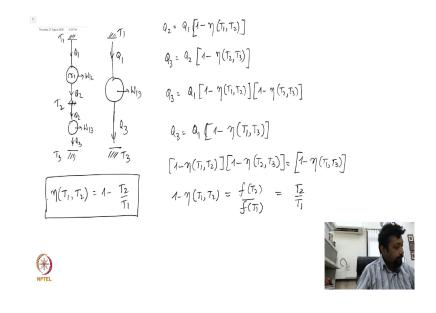
For the second engine so let us just briefly draw this again Q 1 CE 1 does the word W 1 2 Q 2 the second one again takes a heat Q 2 does the work Q 3. So, it does the work W 1 3 and
