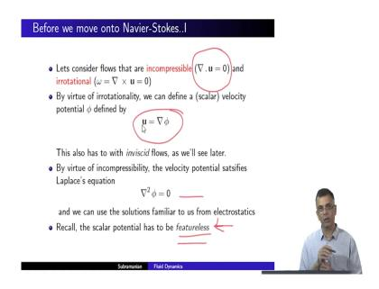
So, this has to do with inviscid flows as we will see later; I just explained this to you. By virtue of incompressibility right; so we already we have already said that u is defined as a gradient of a scalar potential. On top of it we are saying that the flow is in incompressible. In other words the divergence of the gradient which boils down to this Laplacian here is equal to 0 right.
