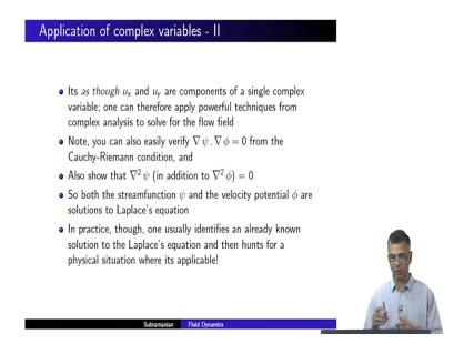
So, I just wanted to point this out and this yeah is as though ux and ui are components of a single complex variable one can therefore, apply powerful techniques from complex analysis to solve for the flow field 2 dimensional flow fields I must emphasize. Although you know a lot of this is done from mathematical convenience its also very relevant to real flows, these are the early days this is how much of the early progress in fluid mechanics was made.
