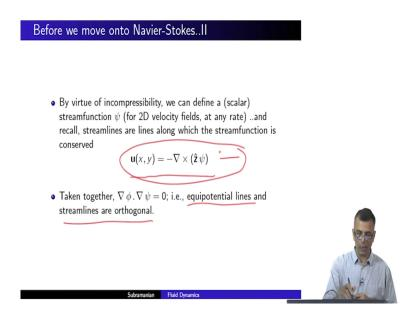
The other thing to remember is that by virtue of incompressibility by virtue of this condition of this condition yeah, you can define a scalar stream function psi, well it is for 2D velocity fields at any rate and recall streamlines are lines along which you know the stream function this is conserved right.
