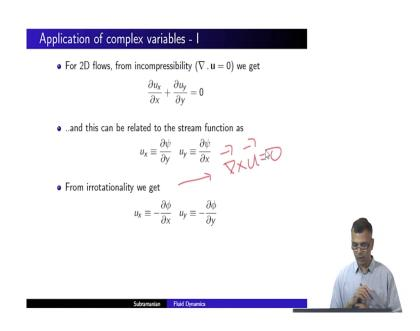
So, and we hinted at this early on you can apply the theory of complex variables to; let us go on and we will see why that is ok. So, for 2 dimensional flows from incompressibility remember we are talking about an incompressible irrotational fluid, incompressible inviscid
