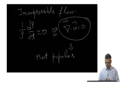
So, let us first consider flows that are incompressible, in other words characterized by you know divergence of u equals 0. Remember that the definition of incompressibility and incompressible flow is 1 for which a Lagrangian observer; an observer sitting on top of a fluid parcel does not discern any changes in density. This is very important to keep this in mind an incompressible flow, is one where; is one where the straight this is equal to 0.
