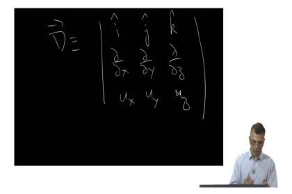
Only when these cross terms are non zero you have a you have a curl that is non zero. If that is not so then the then the flow is irrotational and this paddle wheel will not rotate and what is the situation where the paddle wheel will not rotate? Its one; well where the flow is irrotational or there is really no gradient there is really no sticking between the layers and the flow is effectively inviscid.
