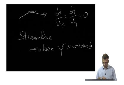
And you can also write it as like that. You can also write a streamline is a streamline is 1, where the stream function psi is conserved; in other words each streamline has a particular value for psi labels a streamline right. So, that is a stream function and taken together in other words taken in other words this equation and this equation taken together gives you this condition and I urge you to work this out.
