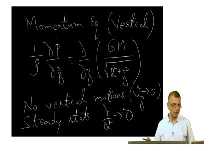
And the vertical component of the Euler equation of the momentum equation. The momentum equation the vertical component looks like 1 over rho dp dz. So, you only have the pressure gradient term and this is equal to d over dz, I will explain what these terms are in a minute.
