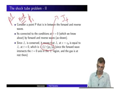
Using conservation of j plus and j minus what we do consider a point P that is in between the forward and reverse waves like we said, this point P. It is connected to the conditions at t equals 0 which we know about by forward and reverse waves.
