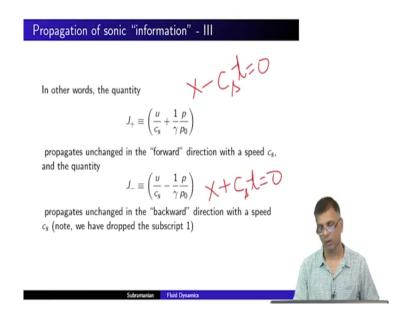
So, this quantity propagates unchanged in the forward direction with a speed c sub s, and this quantity propagates unchanged in the backward direction with the speed c sub s. And note we have dropped the subscripts there used to be a p 1 here or rho 1, there used to be u 1 here, we simply drop that ok just for simplicity.
