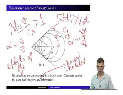
You remember this cartoon, where we found that sonic information in the case where the speed of propagation is larger than the speed of sound propagates in a rather peculiar way. It is only observers within some this thing called a Mach cone the width of which is roughly the half width of the cone is something like C s over V ok. So, it is only observers within this Mach cone who can who receive sonic information and observers outside the Mach cone do not receive this information.
