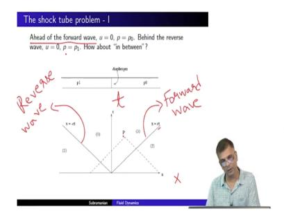
So, you see information propagates at the sound speed right. And there is no restriction on which direction you know the information propagates in. It can propagate to the right and also to the left. In other words, there is a forward wave as well as a reverse wave right. So, the thing is ahead of the forward wave, the information the diaphragm is ruptured has not yet reached ok.
