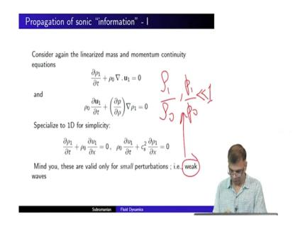
So, these two equations start looking like this. In other words, this is this and this is this that is all right. So, this is c sub s square and we said that nabla rho 1 is simply d rho 1 dx and that is it right. So, this is the linearized mass continuity equation and this is the linearized momentum continuity equation in 1D. Mind you these are valid only for small perturbations very important.
