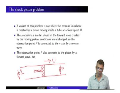
Now, a variant of this problem is one where the pressure imbalance is created by a piston. So, instead of a diaphragm, what you have is a piston. And the piston is moving inside the tube at a fixed speed U ok. So, what you have is a piston. So, you have the same shock tube right. And as before you have p 1 and p naught, the only difference being the piston is moving at a velocity U, this piston is moving at a velocity U. And what happens? Same question, we are asking right.
