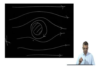
So, you recall the potential flow around a cylinder, you recall this. This is what the flow look like right yeah and around a balls yeah and so like so with the and by the time you reach you are very far away it is as good as straight. Now there is no circulation here; if for some if on top of this I just because I say so let me impose a circulation, in other words let me impose a streamline that looks like this.
