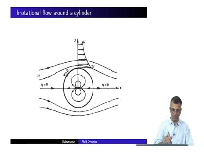
So, what we now saying is that the time rate of change of vorticity is 0. In other words the circulation this quantity K is conserved right. So, circulation is conserved in an inviscid barotropic fluid also importantly it is true only for situations where either the body force is absent or the body force is can be described using a conservative potential ok. That is not written here, but I want to keep I want you to keep that in mind firmly.
