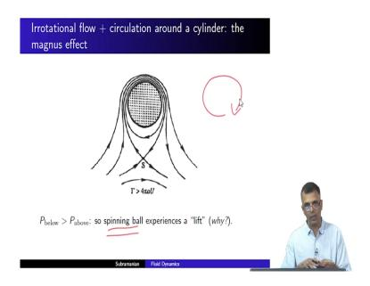
So, now I have mentioned the word spinning ball. This obviously, has to do with the fact that I have included a circulation here right. Now, although we are talking about an inviscid flow right, lets for a moment think about a real life situation where the viscosity is not negligible.
