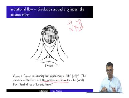
The direction of force is perpendicular the direction of the lift is perpendicular to the rotation axis. The rotation axis as you know is inward like this into the plane and as well as a local flow ok. This is very similar to Lorentz forces which are you know this kinds of very similar to that in electrodynamics.
