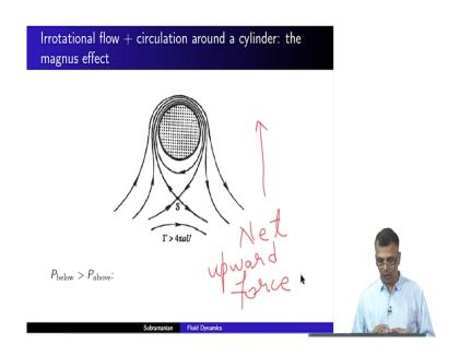
So, as a result of the fact that this lower velocity here as opposed to here, the pressure below will be larger than the pressure above yeah. In other words there is a net upward force in this kind of a situation right. Where, what kind of a situation are we talking about?
