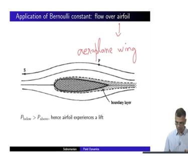
Let us go to another nifty result and that is this is flow over an airfoil or essentially an aeroplane wing, why does an aeroplane wing experience a lift? Ok. This is how this is the fundamental principle around which aeroplanes are designed and this is a rather simplistic way of explaining.
