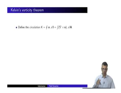
So, we will use this dynamical equation to define something called a circulation and show that for an inviscid barotropic fluid the circulation is a quantity called this. It is a line integral of the fluid over it is a closed line integral and this is something that is conserved and the conservation of circulation will enable us to derive some nifty results that we talked about. So, we will do this when we meet next.
