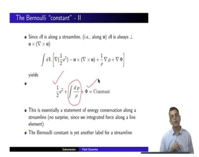
Therefore this term does not matter anymore only this and this matter ok, and what is phi? Phi is simply in this case phi is simply something like gh, where g is a local acceleration due to gravity yeah. So, you have minus gh, let me write this again ok. So, if you plug this in here.
