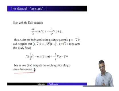
Now, so, throw that away and all we are left with is this where we have made use of this result right. Now, let us integrate this entire equation along a streamline element dl. So, you are not following you are not going along x or along y you are going along a stream line ok, you are integrating along a stream line very important to keep in mind ok.
