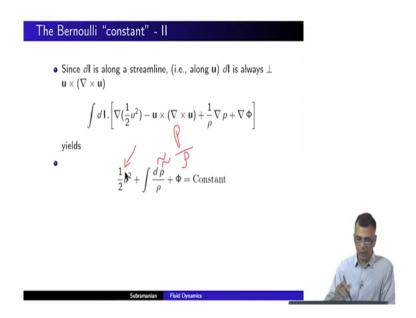
Now, dl by definition dl the you know length coordinate is along a stream line in other words is along u. That is a definition of a stream line right; the stream line is a line that points along u right. Therefore dl is always perpendicular to u cross curl of u, why is that? Well whatever this is curl of u whatever direction it points in you are crossing it with u right.
