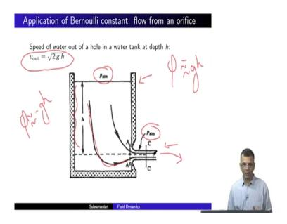
So, here is an application of the Bernoulli constant the application is that of flow from an orifice. So, what you have is a you know a container of water with an orifice here. And you must have you know encountered this many times perhaps specifically from the point of view of a Bernoulli constant must have encountered this problem several times.
