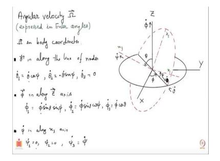
Omega 1 is phi dot sin theta sin psy plus theta dot cost of psy that is correct. Omega 2 is your phi dot sin theta cos of psy minus theta dot sin of psy and omega 3 is phi dot cos theta plus psy dot and this we have, what we have done is the angular velocity has been written in the body coordinates. But you could as well do this decomposition in the space frame, space coordinates in terms of X, Y and capital X, capital Y and Z and that will be also fairly simple.
