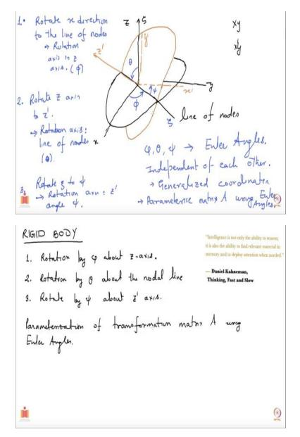
Somewhere here it should be. So, I hope you recall this, I have summarized here, let me write, see this thing. So, rotation by phi about z axis, so you see here the first rotation was about the z axis which was by an angle phi and then you have rotation by theta about the nodal line, so you took the z axis and brought to its new position z prime, by rotating by an angle theta about this line of nodes and then the final rotation was by angle psy about the z axis.
