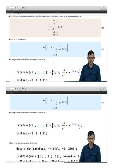
So I do not give you all the steps here. So once again I will load it I probably do not have to do it, because I have loaded it once. Now I have  $dx/dt = v dv/dt = -1/x^2 - \alpha e^{-\beta(x-1)}v$ , x(0) = 1,  $v(0) = v_0$ .
