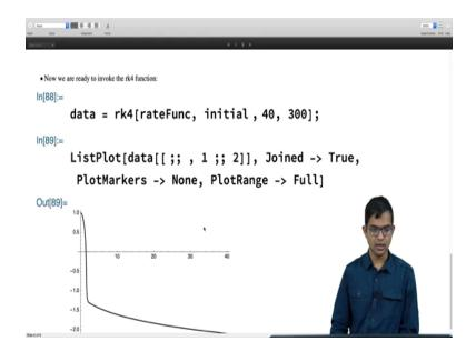
And then I will run this and then I have initial conditions, I have to define the initial conditions. So here I have some room for play. I have my initial other time t = 0 is where I start and x = 1 that is fixed because I started the surface of the earth. But I can pay with different speeds. I can ask myself what will happen if I send my rocket at various speeds and see if there is some critical value which I can extract purely numerically.
