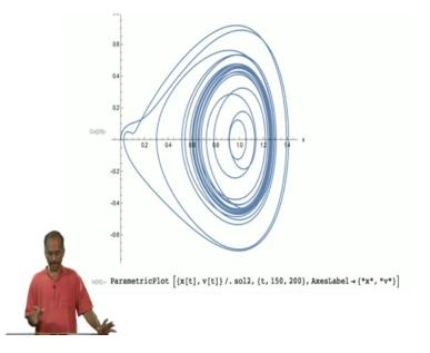
For the choice of parameters that we made, this is what we will get. As I said this is the numerical solution and what is plotted is the phase space plot. So, x axis is the position and y axis is the velocity. So, it already looks like it is very irregular, but that is not so. So initially for first 200 or first 100 time steps when I look at it in phase space, this is
