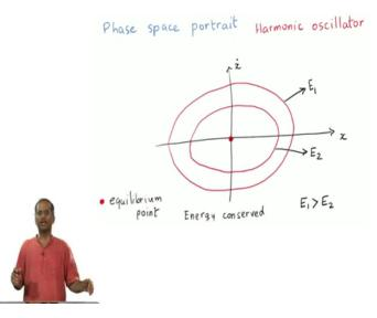
Now let us look at harmonic oscillator again from this perspective. I am going to introduce this idea of looking at it in what is called the phase space. So, on the x axis I have the displacement, on the y axis it is the velocity. So, it is position versus velocity and now I have drawn this for the case of harmonic oscillator standard simple harmonic oscillator.
