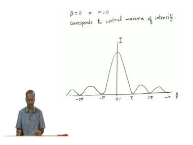
So, in that case  $\beta = 0$ . So, you can put m = 0 in this formula  $\beta$  will be equal to 0 and in that limit this quantity  $\frac{\sin^2 \beta}{\beta^2}$  goes to 1 and what I will have is a maximum; a maxima at the centre m = 0.
