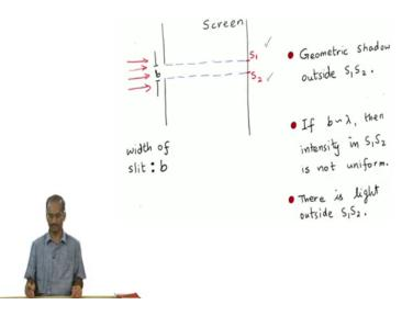
So, let me explain diffraction with the figure that I have here. So, let us assume that there is a light wave front that is coming from the left hand side and it is a plane wave front and it is falling on the slit whose width is b. If light were exactly travelling in straight lines what you would expect is that if I map the slit to a screen a little bit away from the position of the slit, I can mark these two positions  $S_1$  and  $S_2$  as you will see here  $S_1$  and  $S_2$ .
