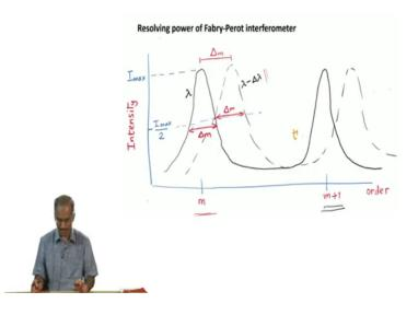
In the sense that when you plot intensity as a function of the interference order the peaks are very sharp for the cases when the reflection coefficient capital R is sufficiently large. But the question that we are now trying to address is what is the resolving power?
