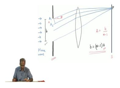
I am going to particularly concentrate on Fraunhofer diffraction of a diffraction pattern arising from a single slit. So, here is a sort of enlarged diagram of the same thing, I assume that the incoming waves are plane and the slit I have has a width b this is the width b which is marked in the figure and this thick dark lines that you see these ones here that is your slit.
