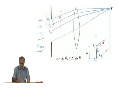
So, I have enlarged this part and shown it here. So,  $A_1$  and  $A_2$  you can see here black line is drawn and that has a width  $\Delta$  the way that we identify a while before. And this is of course, the ray that travels here like this and there is a second ray from  $A_2$  which is originating and travelling in this direction.
