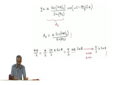
And as you can see when I want to calculate the intensity all I am interested in is this quantity  $A_0$  which is the amplitude and I have extracted this quantity  $A_0$ . So, now I am going to assume that  $\phi$  is small enough. So, I want to know what is  $\frac{N\phi}{2}$  in the first place.
