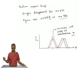
The sodium vapour lamp is made up of two sodium lines D1 and D2 as it is called. What was noticed was that, these fringes which are drawn here; when m is 490 that is the order of the interference is 490, it is really very large order. So, when m is 490, these fringes disappeared and again they appeared when m became 980, this was something that was
