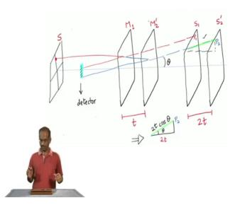
So, here I have the source on the left side. So, that is a screen and I have just taken one point which is denoted by that red dot that you see there. So, S is the screen from where you have, you are getting that extended source and red dot is the one particular point we are monitoring. And my detector is at the position that is shown here. So, as we said, the first thing you will see is this light from the source reaches  $M_1$  and comes back and hits your eye at the detector.
