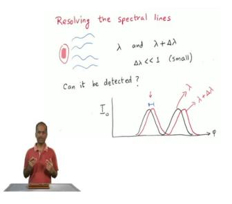
There is an important application of this Michelson interferometer. As I said in determining the wavelength of spectra; but before that there is one important question one needs to answer. Suppose there are, your source of light has two wavelengths which are very close to one another; for instance the sodium line, D2 line is actually made up of two lines which are very close to each other in wavelength or frequency.
