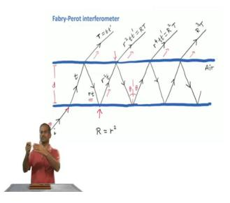
Now, let us look at the Fabry Perot interferometer. So, I have this incident beam which is coming from the lower left end. So, the core part of the Fabry Perot interferometer is this etalon, which allows transmission. So, the incoming beam gets transmitted into the etalon and we assume that the material inside is Air. So, the fraction that is got transmitted is t and at some point.
