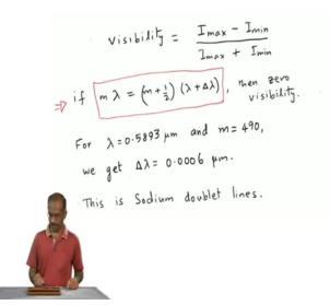
So based on this a quantity called visibility was defined by Michelson himself. So, it is  $\frac{I_{\text{max}} - I_{\text{min}}}{I_{\text{max}} + I_{\text{min}}}$ . You can convince yourself that, if you are using monochromatic light;
