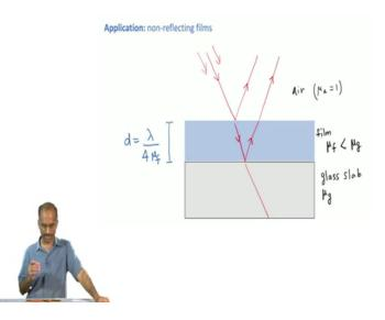
So, I have been using the term glass slabs all the time, because I imagine that we will be doing possibly experiments with glass slabs. So, you can assume at least in small patches that some thin films of possibly oil or of some other material are formed over, let us say water or in general over any other surface.
