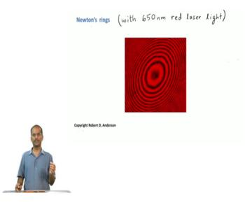
So, here is a result of actual Newton's rings, it was generated with 650 nanometer red laser light and you will see the first thing is that at the center there is a dark spot. So,
