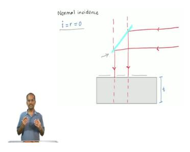
So, first of them is the case of normal incidence. Now what you have is an incoming beam that comes from this right side, as you can see, and I have put a partially reflecting mirror, roughly inclined at 45 degrees. So, what it does is, it allows partial transmission and partial reflection. So, the partial reflection is directed towards the glass slab; whereas, the partial transmission of course, we will go through straight away and nothing we do not worry about that, it just goes through.
