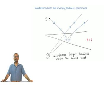
Now, finally, before I leave this subject of glass slab, will also again look at this same problem of wedge shaped glass slab with the light beam as point source, which is at an angle to the top of the glass slab. So, here is your source of light, *S* and you have a beam which comes and hits the top surface of this glass slab, which has the shape of a wedge and the glass slab as usual has refractive index  $\mu$  assumed to be, assumed to have a value greater than 1.
