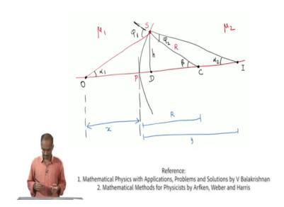
Unless, there is a reason for the ray to get refracted within a given medium, where the refractive index is a constant, the ray basically traces a straight line. So, which means that I need to worry about ray deviating from the straight line only at points where refraction takes place.
