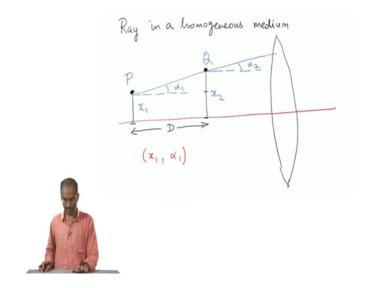
So, here I have written the product of two matrices capital A and capital B. The basis of treating rays using matrix methods is actually shown in this diagram that I have just drawn. The ray between P and Q or even a little further can be described by the quantity
