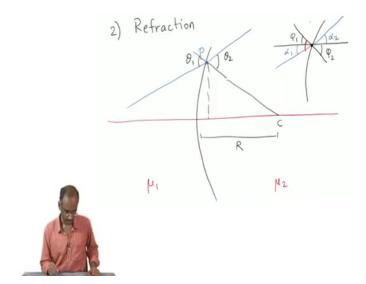
Here I have a refracting surface like I have shown in black line and red line represents the axis; let me call it by P, the point at which refraction of the ray takes place.
