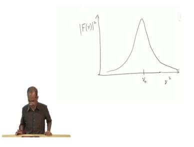
So, this is how the function would look like, the Fourier transform of a function whose amplitude is exponentially decaying. So, this was my f(t) and here I have plotted the power spectrum. The peak occurs when  $\nu = \nu_0$ . In other words, it is equivalent to saying that  $\nu_0$  or the frequency  $\nu_0$  contributes most to this function, all other frequencies contribute relatively lesser and there is a decay around  $\nu_0$ .
