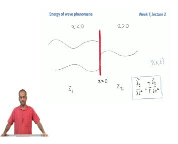
Welcome, this will be the 2nd lecture of 7th week. So, here is a picture that summarizes what we did in the last module. So, our standard scenario is that the wave comes from the extreme left and hits the boundary at x = 0. So, there is change of media a part of the wave gets transmitted into the second medium and another part gets reflected back into the first medium. So, we can identify an incident wave; for instance as it is shown in this schematic diagram.
