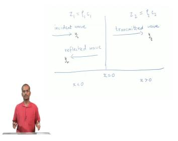
So, there is an incident wave, which I call  $y_i$  yagain is the displacement and this displacement of the particles that constitute the wave would be a function of both space and time. So,  $y_i$  will be a function of x and t. So, there is a transmitted wave which we have designated as  $y_t$  and then there is a reflected wave which we have called  $y_r$  and importantly these two media one that is x < 0 and x > 0 they are characterized by different values of impedances.
