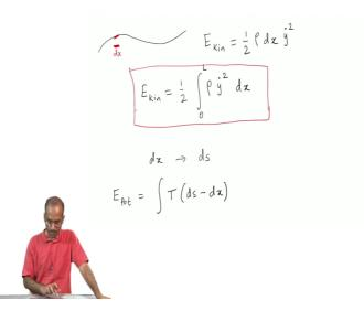
So, let say that, I have this string and I am looking at some small segment. Whose length is dx. So, in such a case the kinetic energy would be mass times velocity square. So, that is half mass here is the linear density multiplied by dx times velocity square, which is this the particle velocity. Now, I want to calculate the energy over a larger length in which case I could write  $E_{kin}$  to be. So, this is my expression for kinetic energy.
