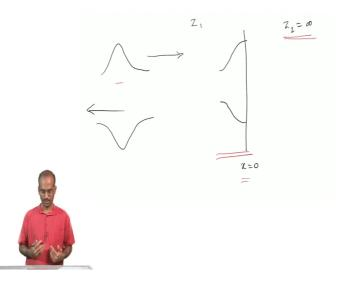
So, pictorially what we have is that there is an incoming wave as you can see which is this. It comes and hits the boundary here at x = 0 and what I have tried to show here is when part of the wave has already been reflected of the boundary. And here I have assume that  $Z_2$  is infinity which means that second medium offers infinite resistance to
