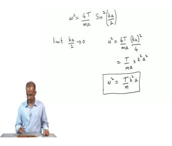
Now, let us consider the limit when  $\frac{ka}{2}$  is small or when k is small really, a is a constant, so the only variable there is sort of k and let us take the limit  $\frac{ka}{2} \rightarrow 0$ ; in that case in this limit the normal mode frequencies would be  $\frac{4T}{ma}$ . So,  $\sin \theta$  can be replaced as  $\theta$  in the limit of  $\theta$  being very small, so this would give me  $\frac{(ka)^2}{4}$ .
