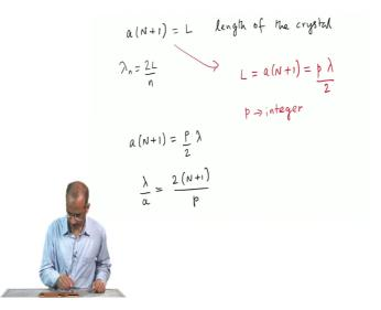
To go further we also know that a(N + 1). So, assuming that we have N atoms in the crystal, a(N + 1) = L which is the total dimension or length of the crystal, we can directly equate this using this condition. So, remember that this is the condition that we had obtained in the previous module for the allowed wavelengths of standing waves. Here the current problem that we are doing is equivalent to a system of N atoms, which are arranged in a linear lattice.
