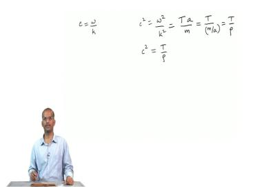
So, if I go back to my expression here, I can write an expression for  $\frac{\omega^2}{k^2}$ . So,  $c^2$  would be  $\frac{\omega^2}{k^2}$  and that would be equal to  $\frac{Ta}{m}$ , which would be equal to  $\frac{T}{\rho}$ . So, the phase velocity in the limit when  $\frac{ka}{2}$  is small would be  $\sqrt{\frac{T}{\rho}}$ . Now, let us go to the other case when  $\frac{ka}{2}$  is
