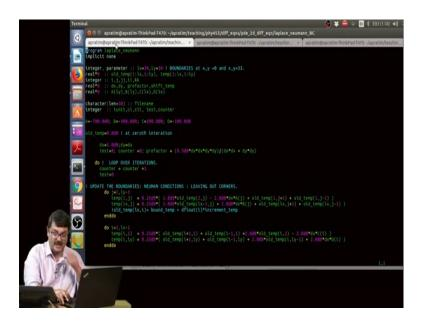
And this is the program Laplace Neumann and here I specify the lattice sizes L x equal to 34 just as the previous case and L y equal to 34 just as the previous case. Now note I have four arrays called A l y, A l y, C l x and D l x. So, these are those A B C D which I specify at the boundaries right, those are the amount of heat current and that you specify at the boundaries and the rest of it is basically very similar to the previous code.
